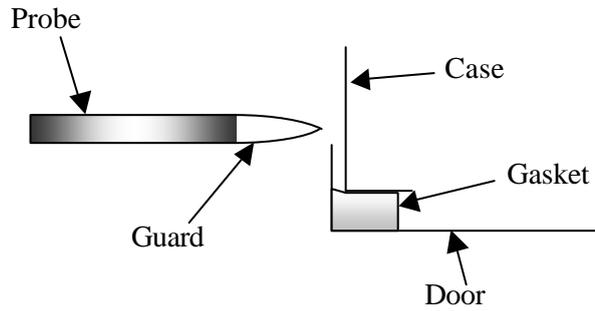
**Position 1 - Probe at right angle to side of boiler**
