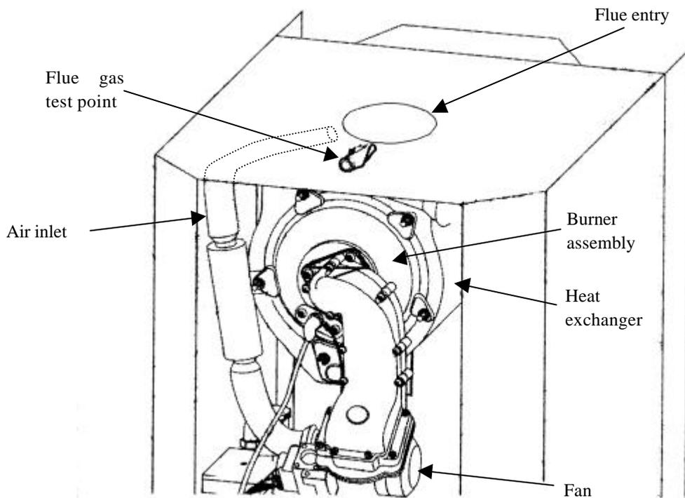
Figure 3 – Ecomax – drawing of boiler
