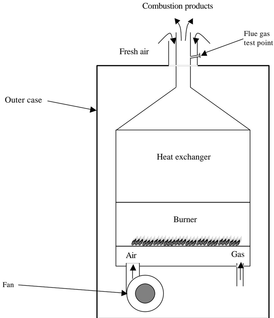
Figure 2 – Schematic diagram of flow through Envoy and Ecomax boilers
