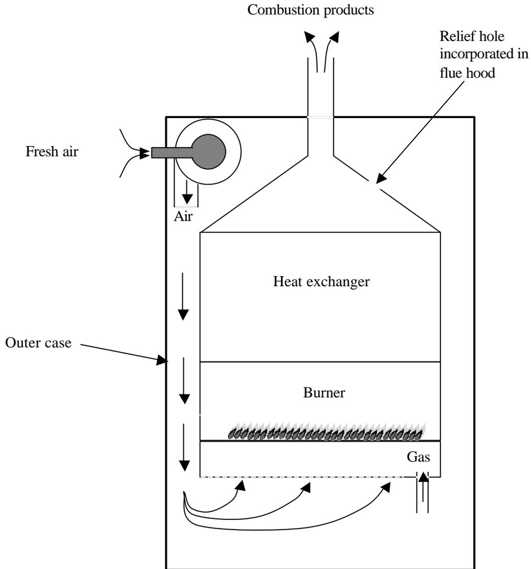
**Figure 1 - Schematic diagram of flow through Netaheat boiler**
