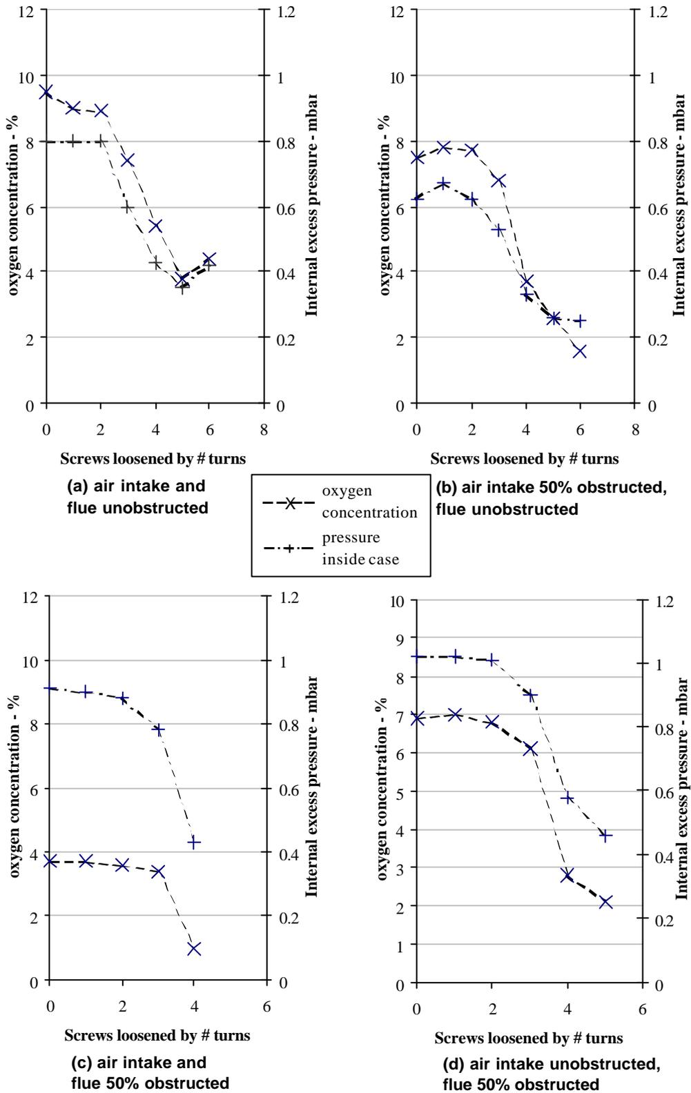
Figure 13. Flue gas oxygen concentration and internal pressure in Netaheat boiler
