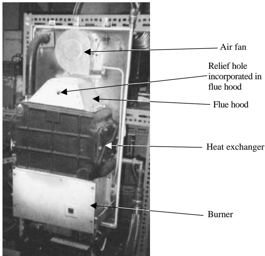
**Figure 7 - Netaheat – photograph of boiler**
