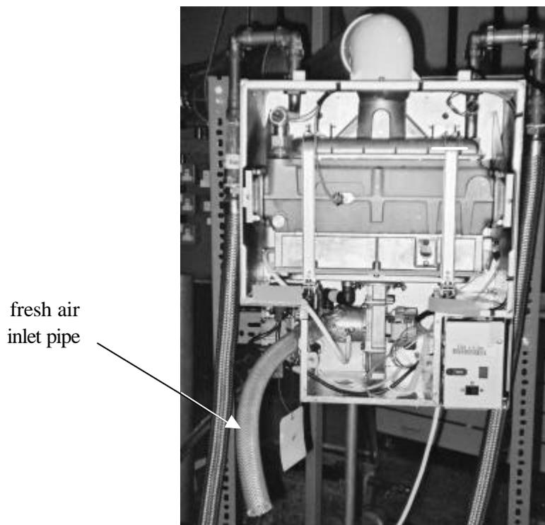
**Figure 8 Envoy – photograph of boiler fitted with external air inlet**
