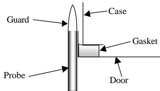
**Position 2 - Probe from front of boiler**
