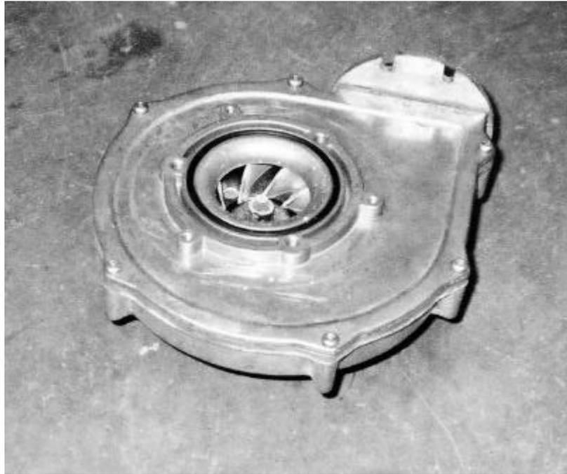
**Figure 10. Photograph of fan from Potterton Envoy, showing deposits on fan rotor after use of smoke pellets**
