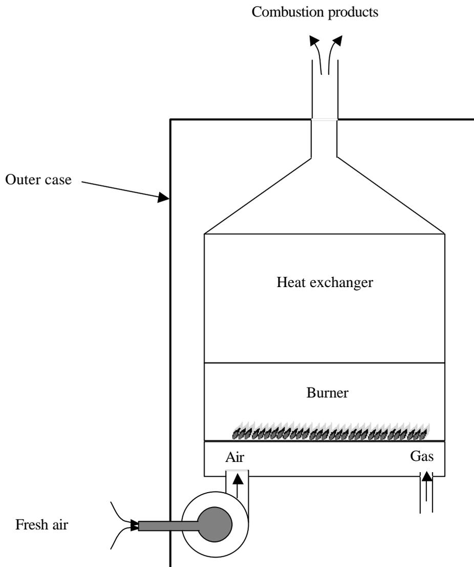
Figure 9 - Schematic diagram of flow through modified Envoy boiler
