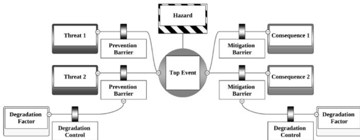
Figure E1. Bow-tie diagram structure 3
