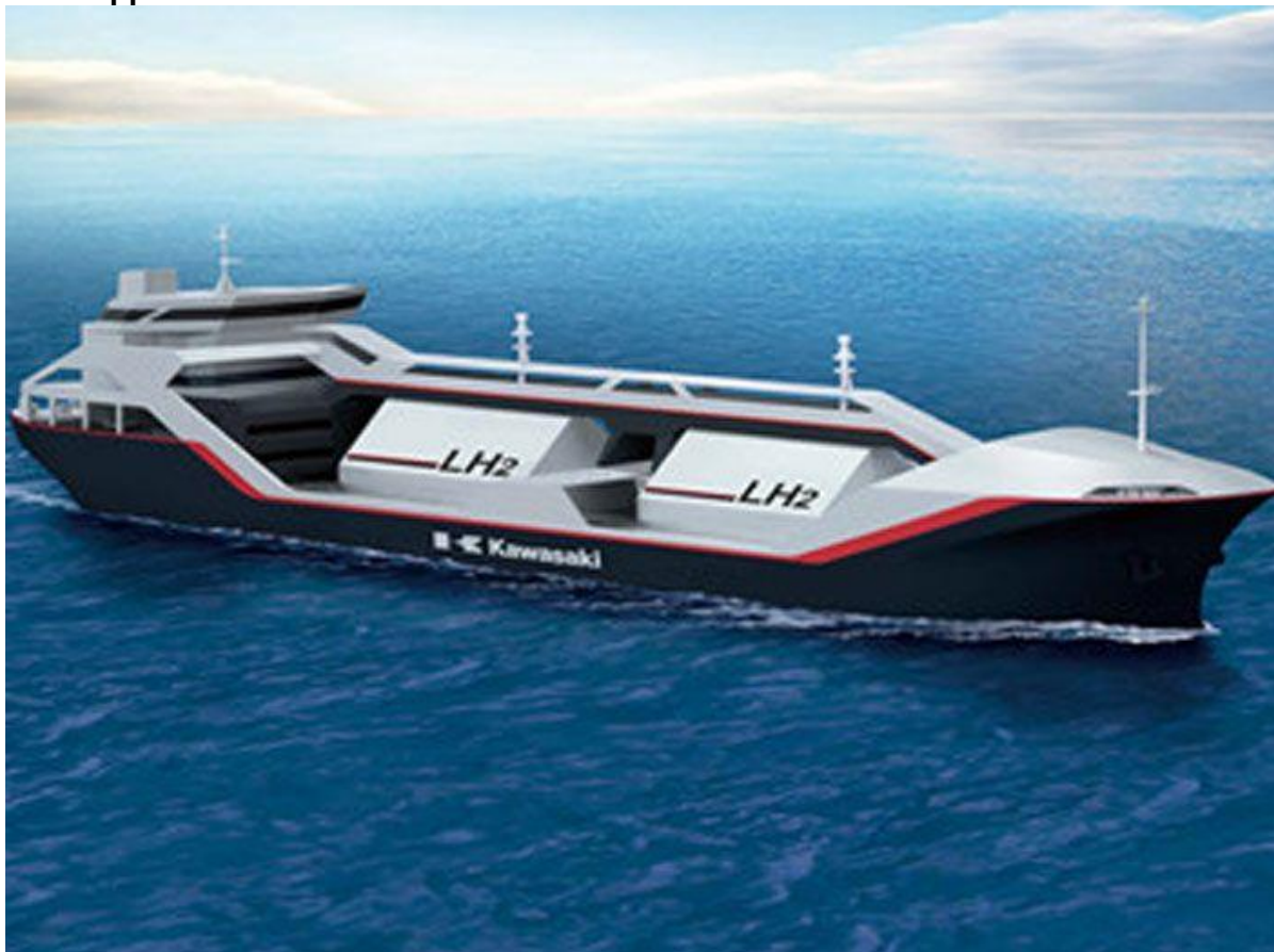
Figure 3.13 Maritime application - artists impression of LH2 transport ship (photo source: Kawasaki Heavy Industries)
