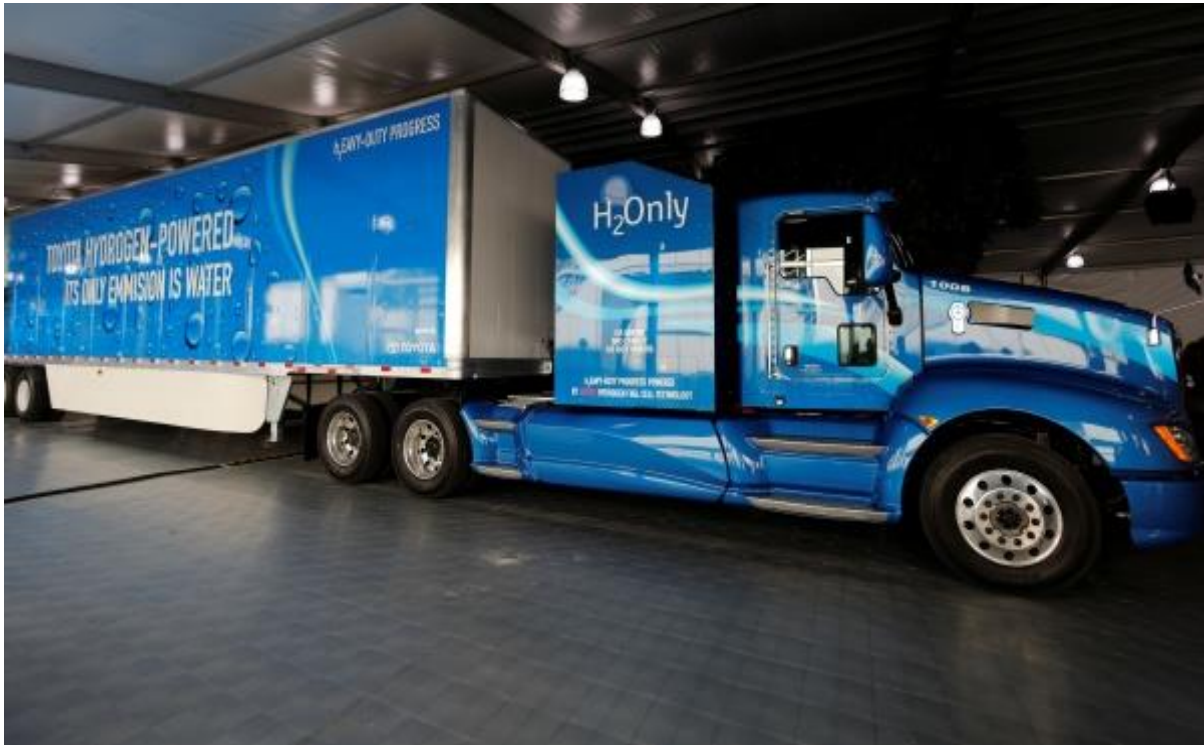
Figure 3.11 LH 2 heavy duty truck application (photo source: Nikola)
