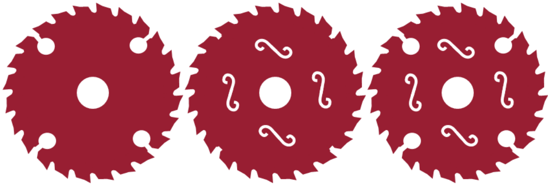
Figure 2 Circular saw blades illustrating: Left: Segmental cut outs, Middle: Spiral cutouts and Right: both segmental and spiral cutouts
