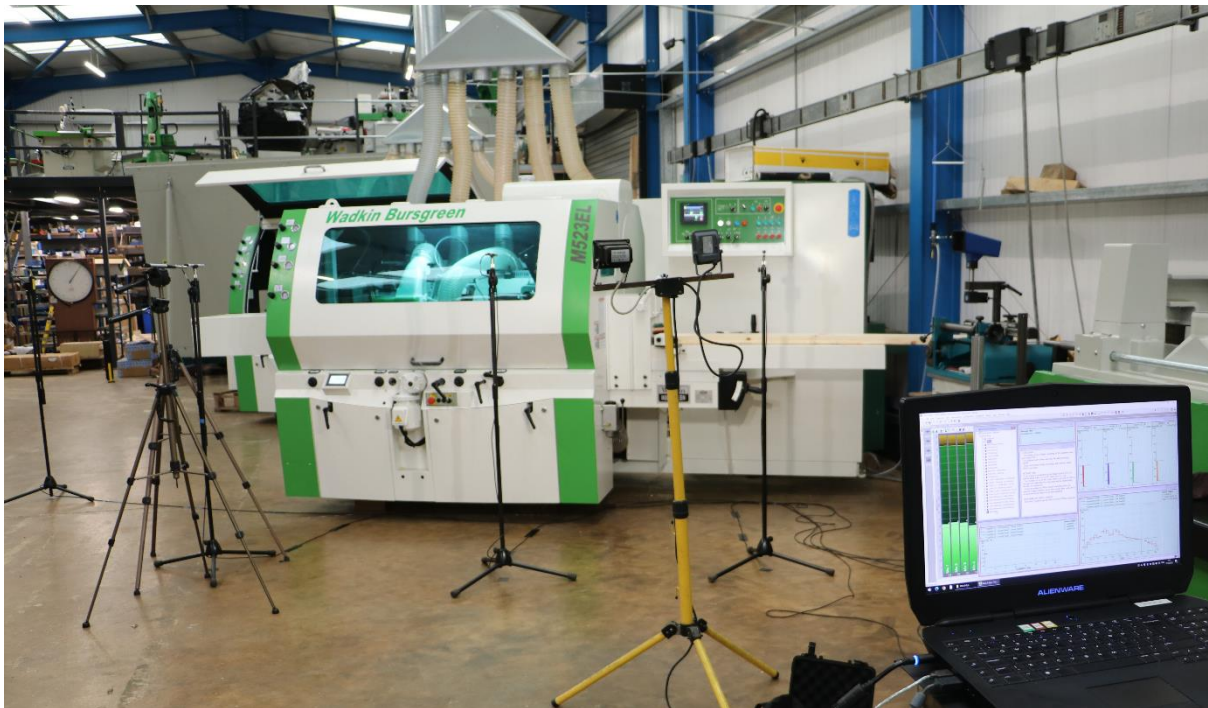
Figure 8 Wadkin Bursgreen MS525EL-5 with the enclosure lid down (photo IMG_2284.jpg), also showing microphone positions and wood ready for cutting on the in-feed.
