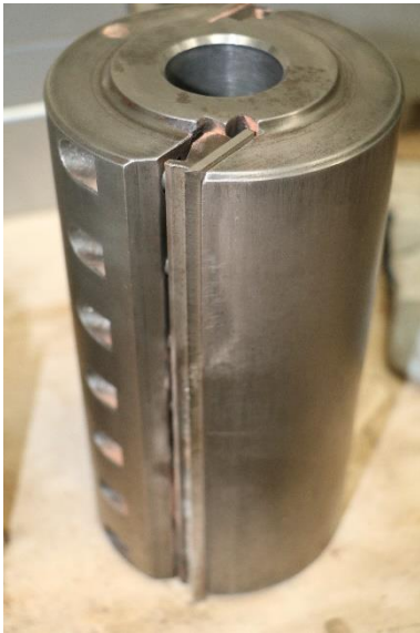
Figure 11 Wadkin straight cutter blocks (Left: 230 mm horizontal cutter, photo IMG_2309.jpg. Right: 130 mm vertical cutter, photo IMG_2311.jpg)
