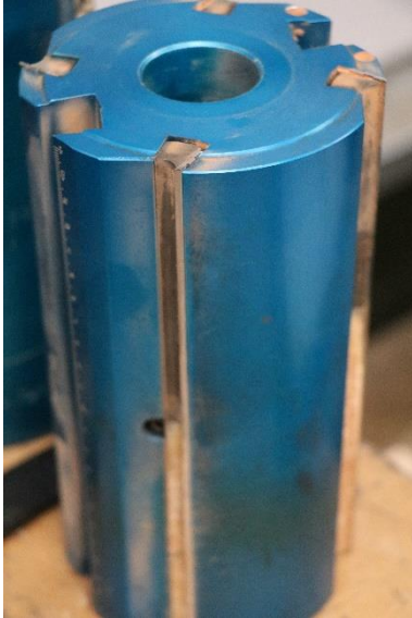
Figure 13 Stark Plannex horizontal aluminium cutter blocks (Left: 230 mm horizontal cutter, photo IMG_2251.jpg. Right: cutter #4 in machine, photo IMG_2250.jpg)
