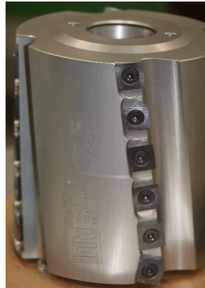
Figure 12 Leitz HeliPlan® helical cutter block (Left: 230 mm horizontal cutter, photo IMG_2298.jpg. Right: 130 mm vertical cutter, photo IMG_2295.jpg)
