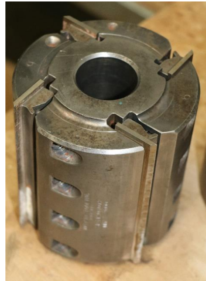
Figure 11 Wadkin straight cutter blocks (Left: 230 mm horizontal cutter, photo IMG_2309.jpg. Right: 130 mm vertical cutter, photo IMG_2311.jpg)
