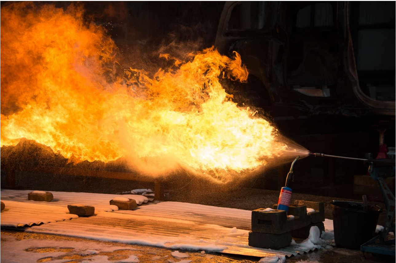
Figure 5: Hydraulic fluid (mineral oil) spray fire
