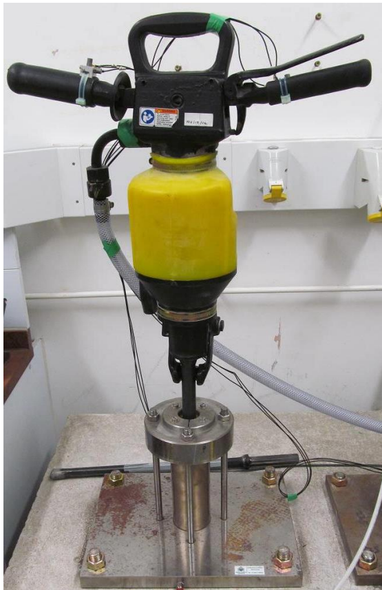
Figure B.4. Riveting hammer showing the front and rear hand positions, with the bucking bar (right)
