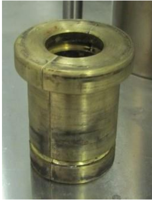
Figure 2a. Collar for new dynaload to BS EN ISO 28927-10:2011
