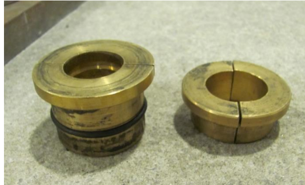
Figure 2b. Collars for old dynaload; 1 mm clearance (left) and 3 mm clearance (right)
