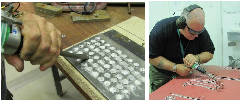
Figure 4. (a) Rivet busting (left) and (b) panel ripping (right)
