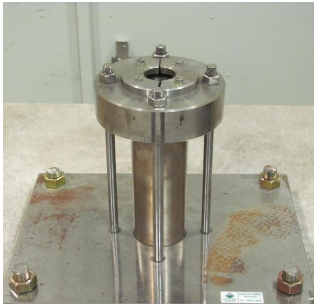
Figure 1b. HSE type 1 40 mm dynaload to BS EN ISO 28927-10:2011
