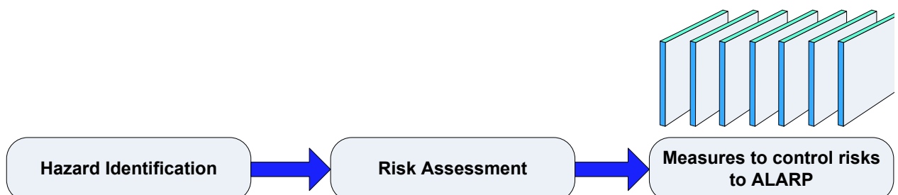
Figure 3 Sequence of analysis to determine the appropriate control and mitigation measures for major hazards
