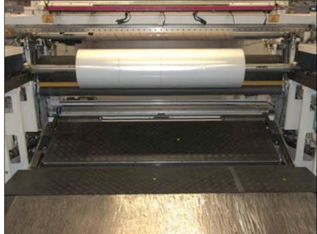
**Figure 4** Example of pressure mat zone 1 protection
