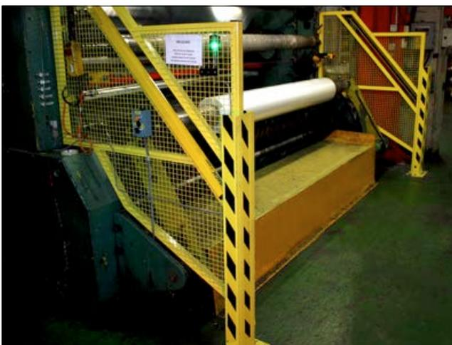
**Figure 3** Example of ESPE zone 1 protection
