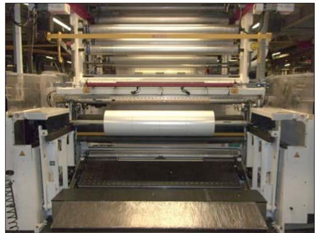
**Figure 1** Drive roll arrangement
