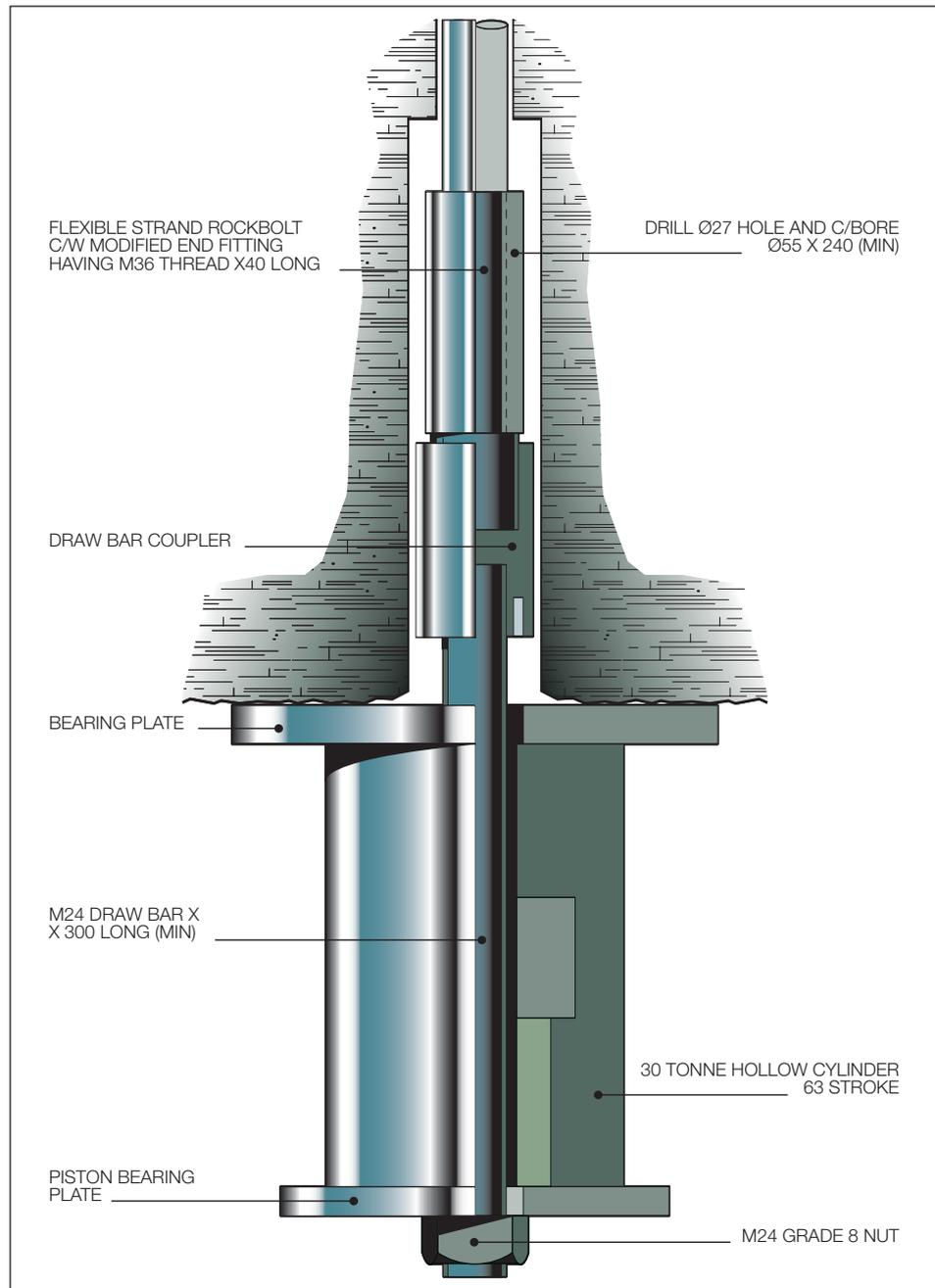
**Figure 2** Arrangement for pull testing of a flexible bolt
