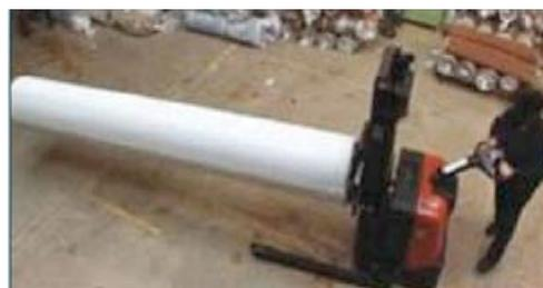
**Figure 2** Pedestrian-powered truck with boom attachment
