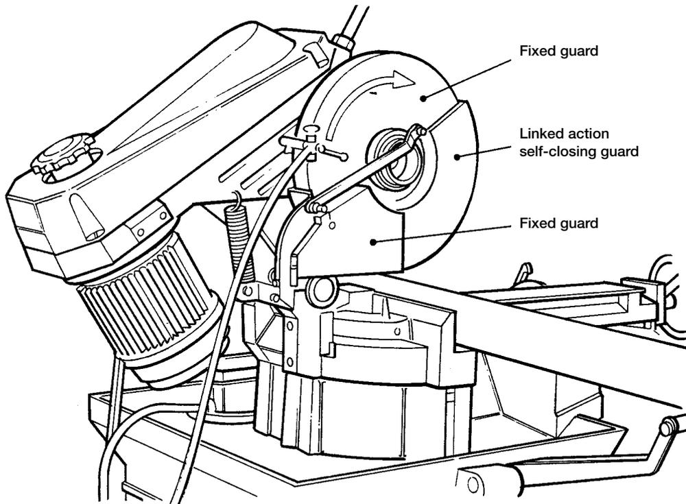
**Figure 1** Manually fed, pivoting-head, metal-cutting saw
