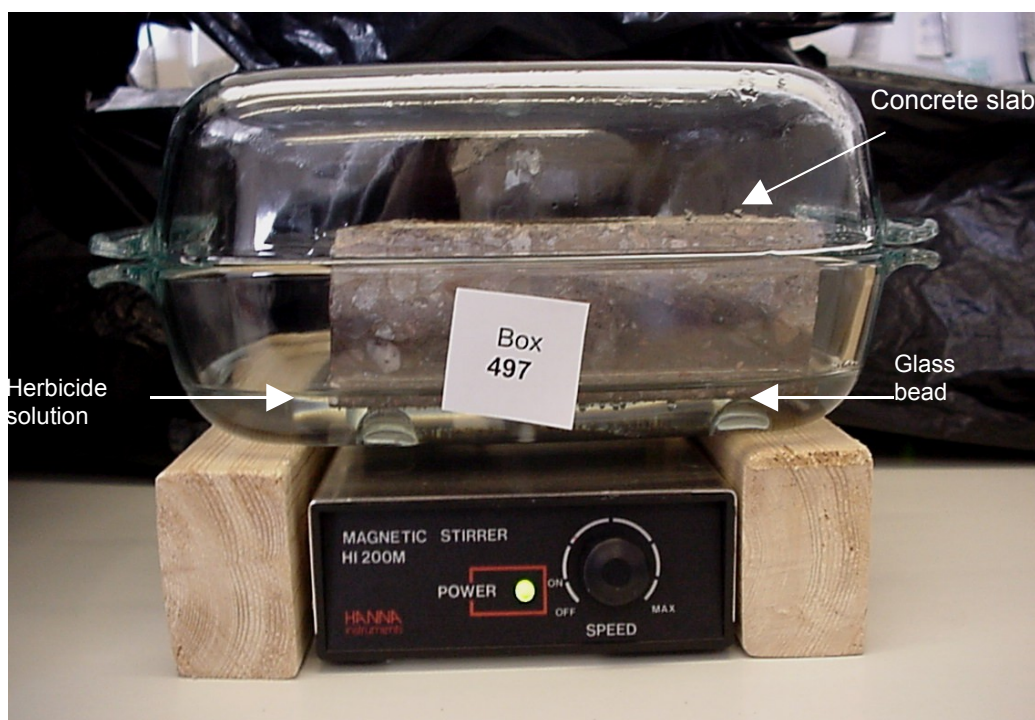
Figure 1 Experimental apparatus for the sorption study
