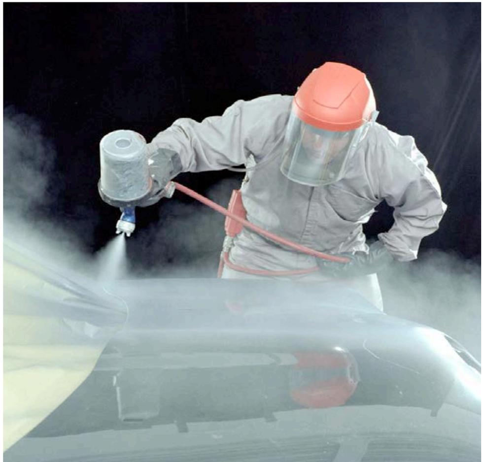
**Figure 4** This worker is spraying paint containing isocyanate. The fine spray, not normally seen with the naked eye, is shown up with the use of 'Tyndall illumination'. Skin and inhalation exposure to isocyanates has the potential to cause skin allergies and asthma. The right controls should be used to minimise exposure
