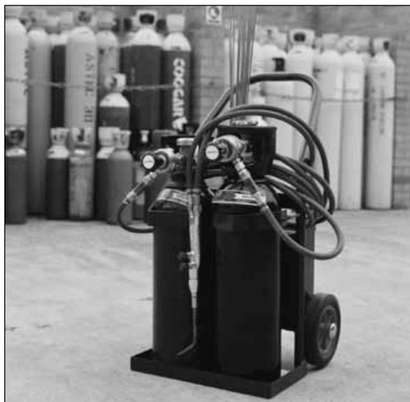
67 Manual handling of heavy gas cylinders easily results in accidents causing back strain, trapped fingers, bruising to hands or feet, etc. The aim should be to avoid the need for anyone having to move gas cylinders by hand. Where this is not reasonably practicable, employers should carry out an assessment of the handling operation in accordance with the requirements of regulation 4(1)(b)(i) of the Manual Handling Operations Regulations 1992<sup>52</sup>. The risks indicated by the
