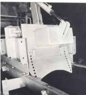
**Figure 11** Transfer point receiving hopper with adjustable guillotine door
