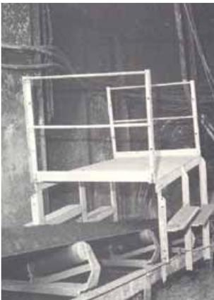
**Figure 8** Access bridge over conveyor
