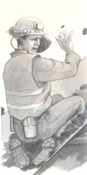
**Figure 18** Potential danger of manriding with mineral on steep gradients
