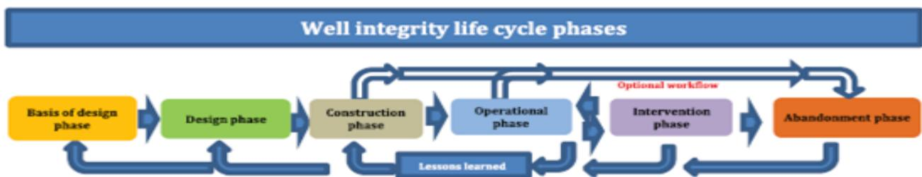
This inspection guide is concerned with the operational phase. Wells will spend the vast majority of their life in the operate phase therefore this guide targets the greatest cumulative risk. The design phase, construction, intervention and abandonment phases are inspected through the Well Notification process.
