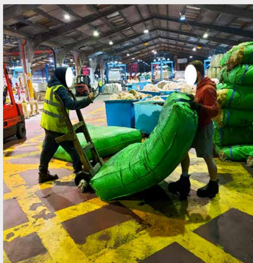
Wool sheets manually handled with sack barrow
