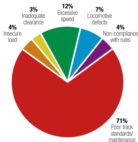
**Figure 4a** Primary cause of derailments on track 1986 to 1988
