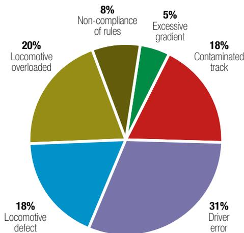
**Figure 6a** Primary causes of runaways 1986 to 1988
