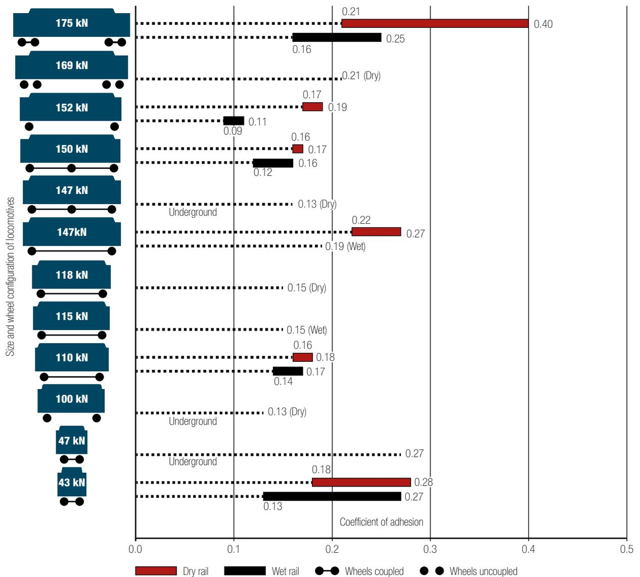
**Figure 8** Variation in coefficient of adhesion of underground locomotives
