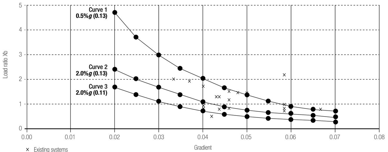
Figure 10 Effect of load/gradient on deceleration of locomotives with uncoupled axles
