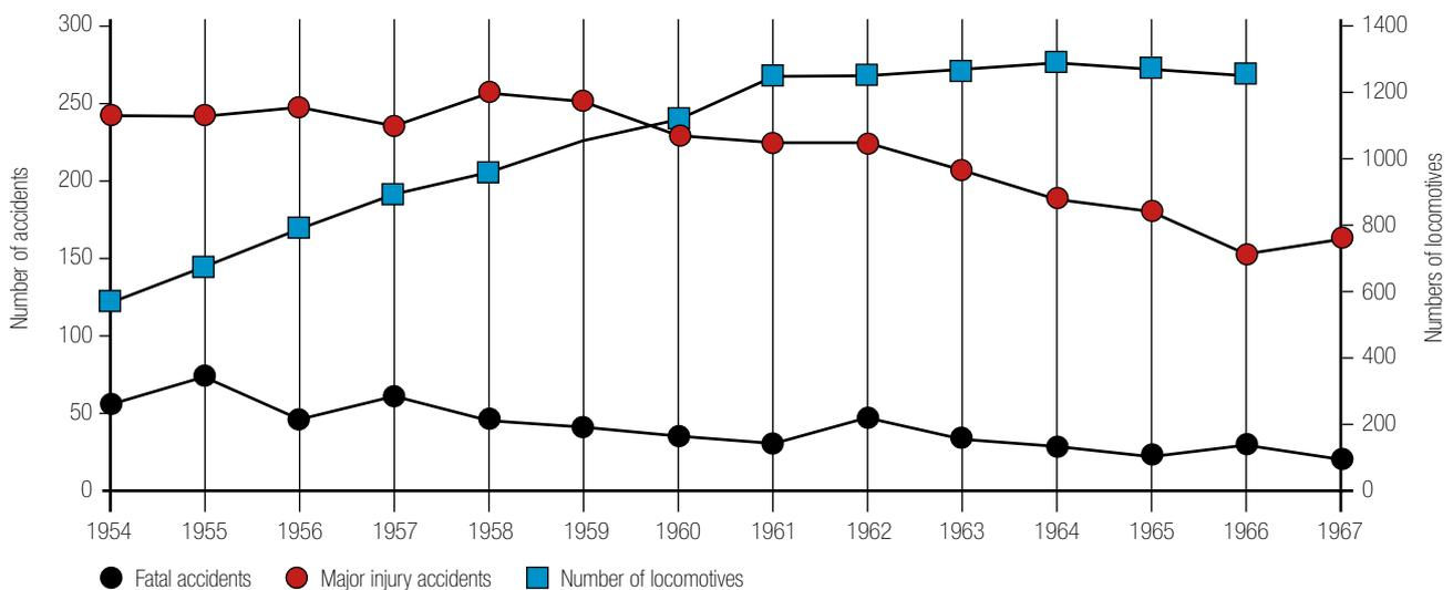
**Figure 1** Underground mechanical haulage - fatal and major injury accidents 1954 to 1967 (Figures supplied by British Coal)
