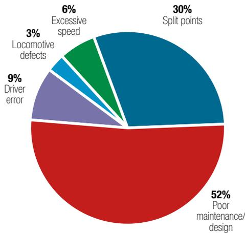
**Figure 5a** Primary cause of derailments on points 1986 to 1988
