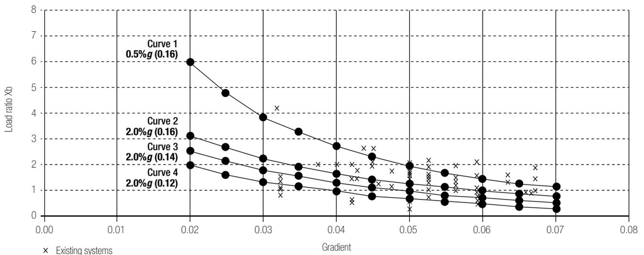
**Figure 9** Effect of load/gradient on deceleration of locomotives with coupled axles
