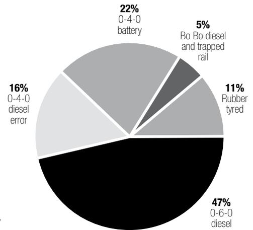
**Figure 5b** Analysis of underground locomotive incidents April 1986 to December 1988
