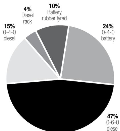
**Figure 4b** Analysis of locomotive types 1986 to 1988
