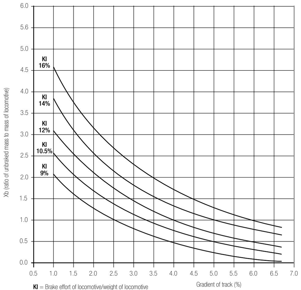
**Figure 11** Graphical method of calculating trailing load for selected operational brake demands to produce retardation of 2% g
