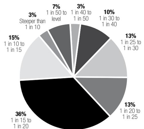
**Figure 6b** Analysis of gradients on which runaways occurred 1986 to 1988
