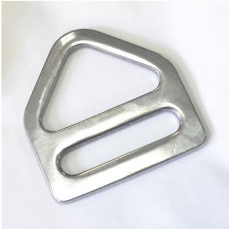
Figure 1 Fall-arrest (single use) attachment - not suitable for multiple loading as harsh angles cause excessive wear to harness webbing
