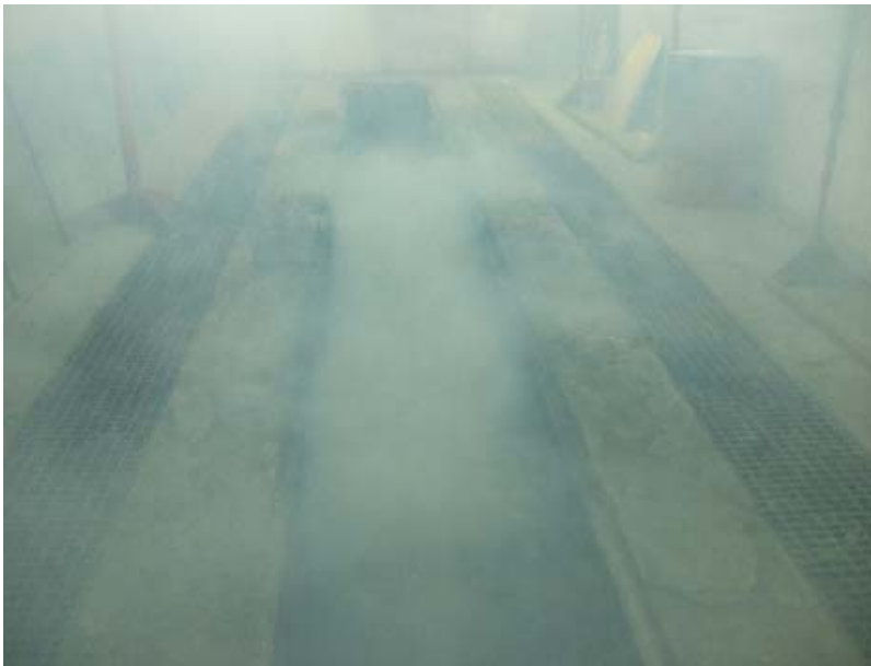
Figure 6. Photograph taken during a smoke test. The smoke clears much slower from an unventilated working pit compared to the rest of the booth
