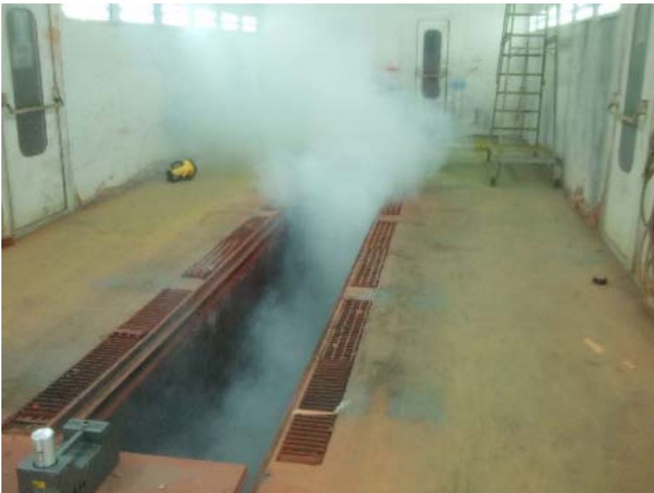
Figure 8. Air movement test using smoke in the working pit of a booth.
