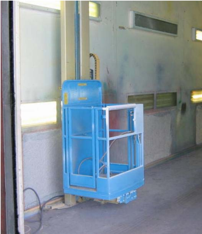
Figure 16. A mobile platform used to access the sides of double decker buses. The platform allows the operator to move easily along the length of the vehicle.
