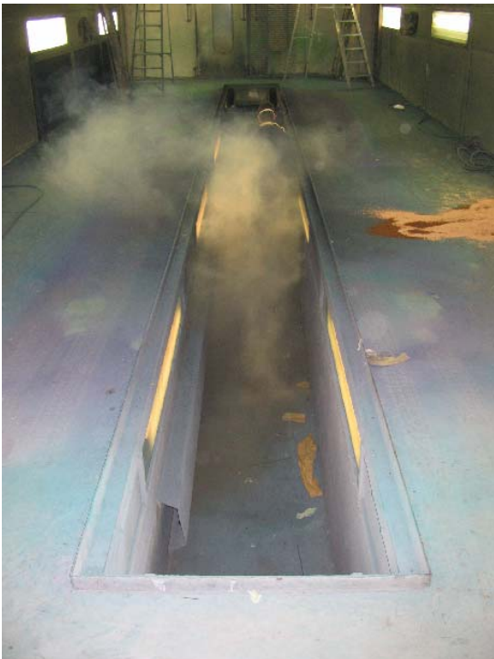
Figure 12. Photograph of the pit being filled by a smoke machine operator while extraction is turned on: as the operator traverses the pit the smoke behind him is rapidly removed from the pit
