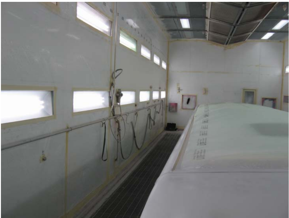
Figure 14. A vehicle lift system in a booth. The vehicle in question is a coach that has been lowered into the floor. The object in the centre of the booth is the coach roof.
