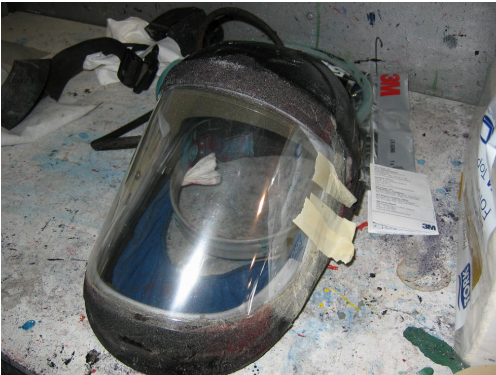
Figure 2. Several visor protectors attached to a visor using adhesive tape
