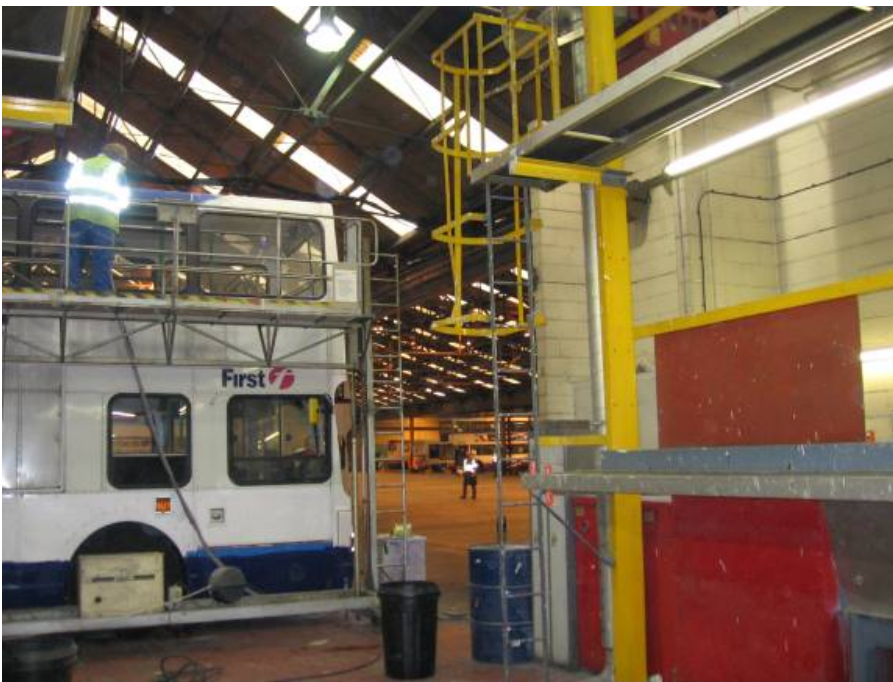
Figure 16. A mobile platform used to access the sides of double decker buses. The platform allows the operator to move easily along the length of the vehicle.
