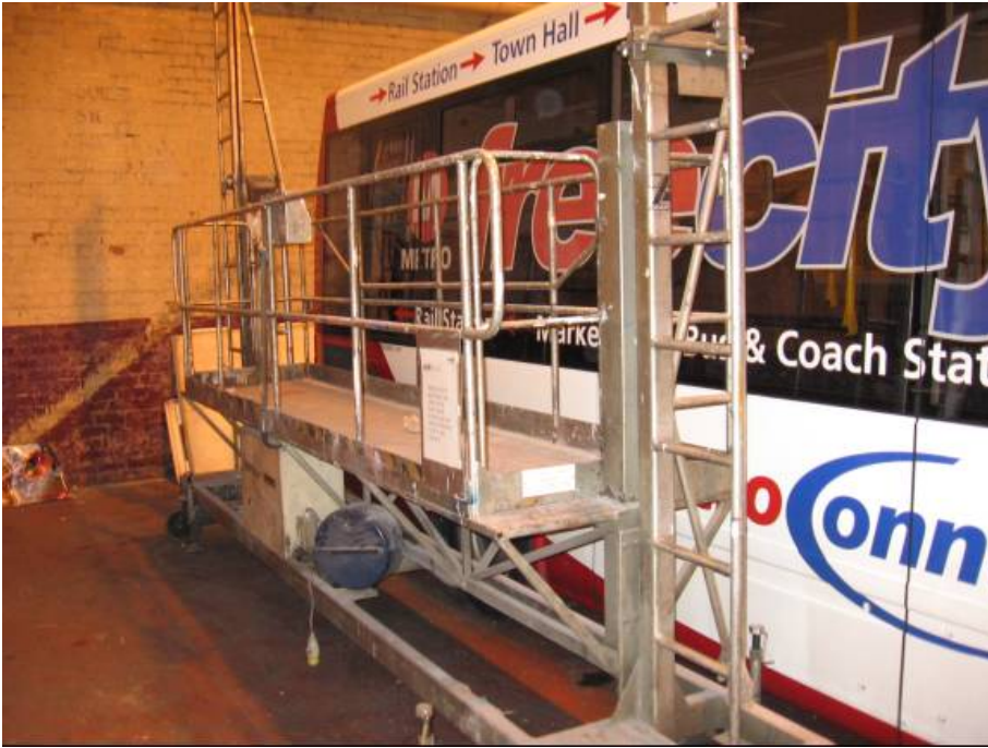
Figure 17. A view of a similar platform to that in Figure 16 in a lower configuration.
