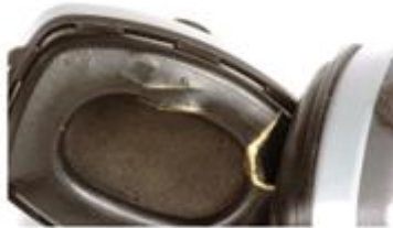
Torn /Burst / Hardened Seals
