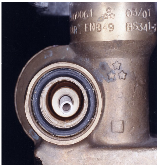
3 Stars and markings on valve with plug removed
