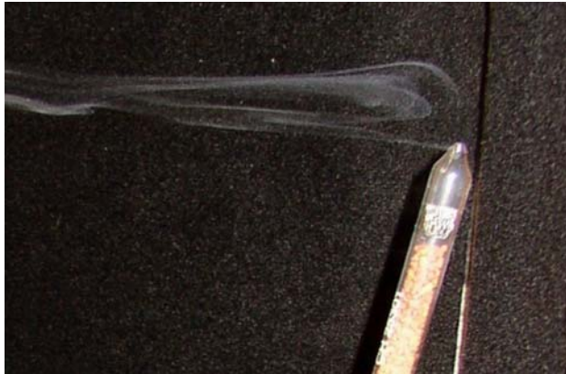
Figure 1. Smoke pencil showing deviation of smoke plume to the left due to a 3mm diameter leakage point.
