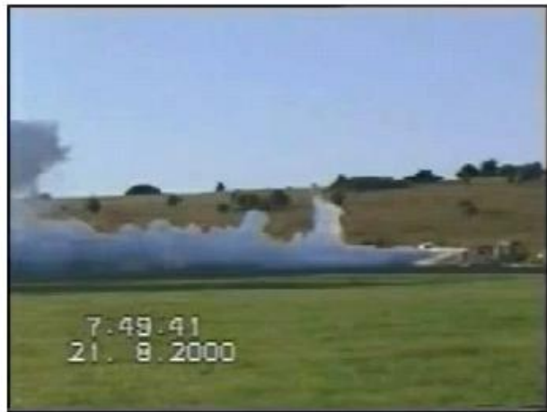
Figure 21, the cloud is seen to have lifted away from the ground. However, this is intermittent behaviour, and the cloud appears to be grounded at this same position for different times. Some of the observed behaviour in trial 12 may be attributed to the effect of atmospheric updrafts and downdrafts in unstable atmospheric conditions, although it might also be influenced by cloud buoyancy induced by HF thermodynamic interaction with atmospheric humidity. In DRIFT the effect of atmospheric updrafts and downdrafts is included as an additional vertical spread on the time averaged plume (based on the probability density model of Weil et al. (1997)), whereas the HF thermodynamics model influences the cloud buoyancy and buoyant rise.
