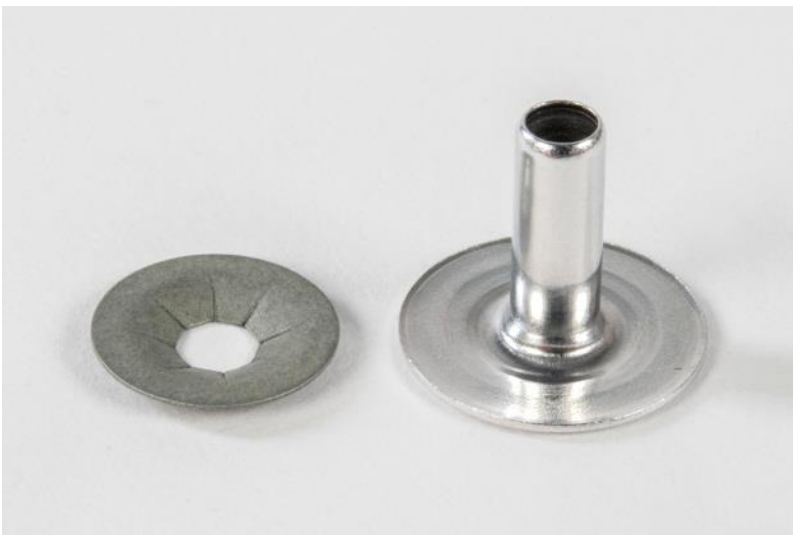
Figure 1 Disposable metal port. The pieces clamp together on either side of the respirator material (image 1703025_020.JPG)
