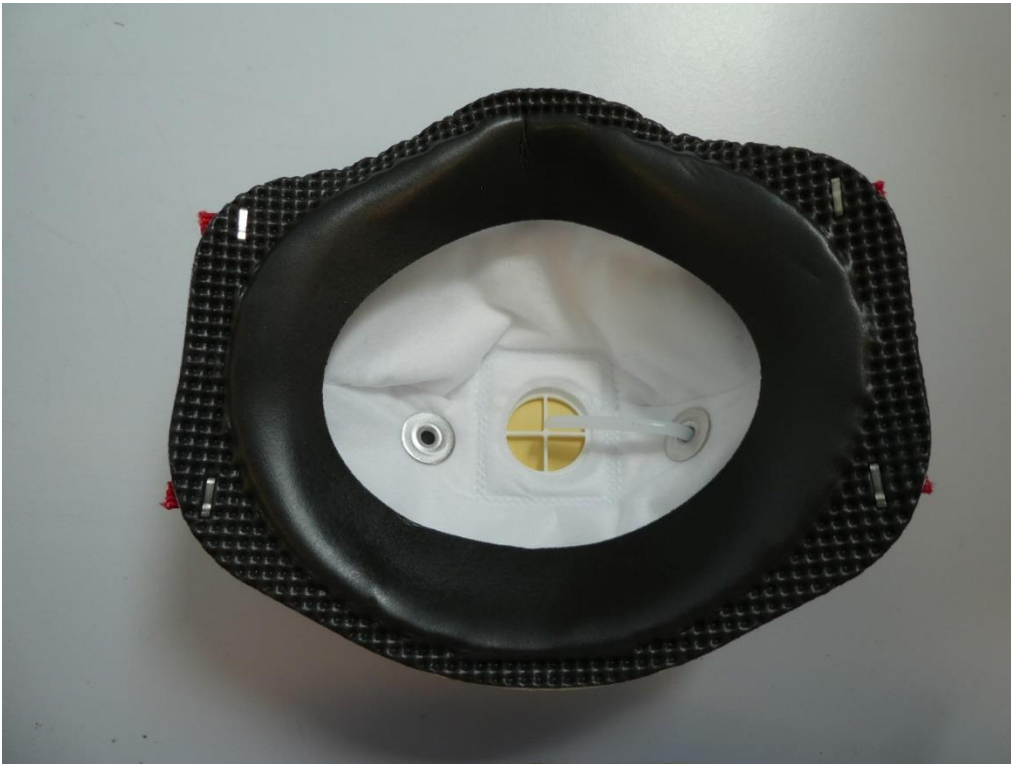
Figure 2 Example of a respirator with a flush and extended port: the flush port is on the left; the extended port is on the right (image P1000066.JPG)
