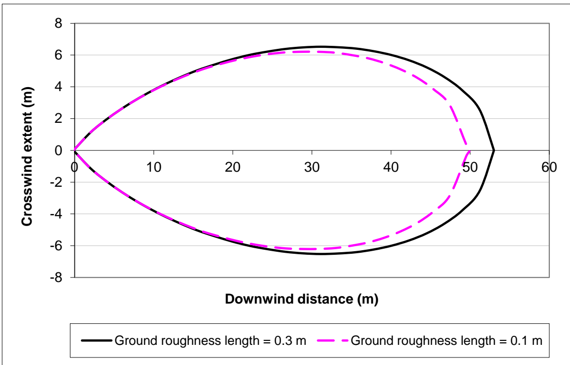
Figure 85 LFL isopleths for a release from a 25 mm hole in an ethylene pipeline in F2 weather for suburban and rural ground surface roughness lengths
