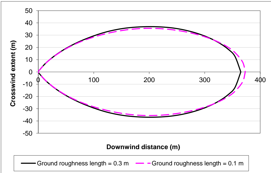
Figure 78 LFL isopleths for rupture of an ethylene pipeline in D5 weather for suburban and rural ground surface roughness lengths
