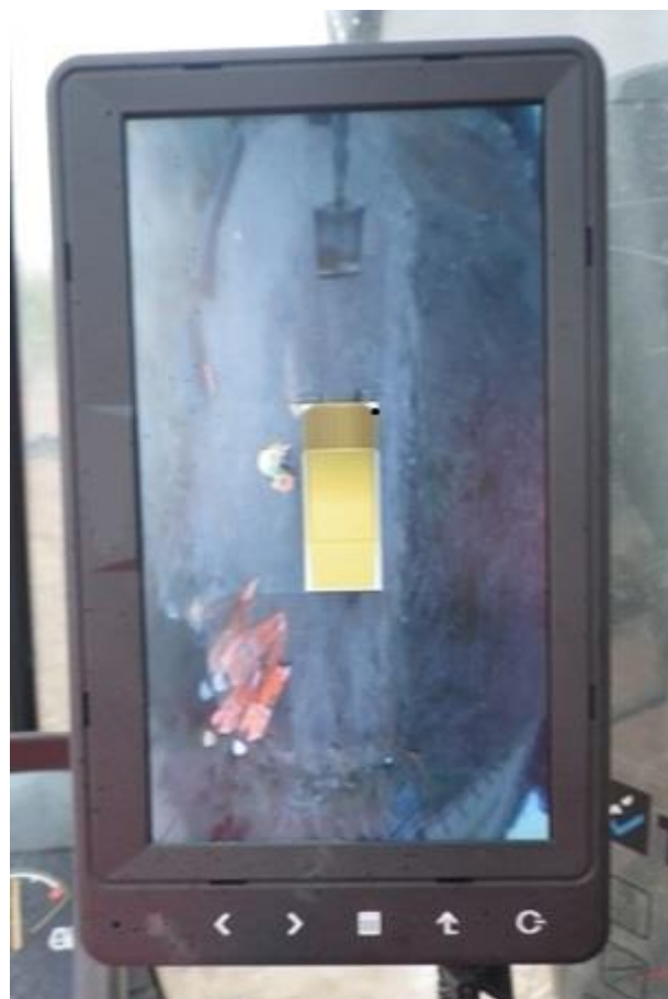
Photograph 1 Example of a monitor display from a camera system, showing a surrounding view for an excavator
