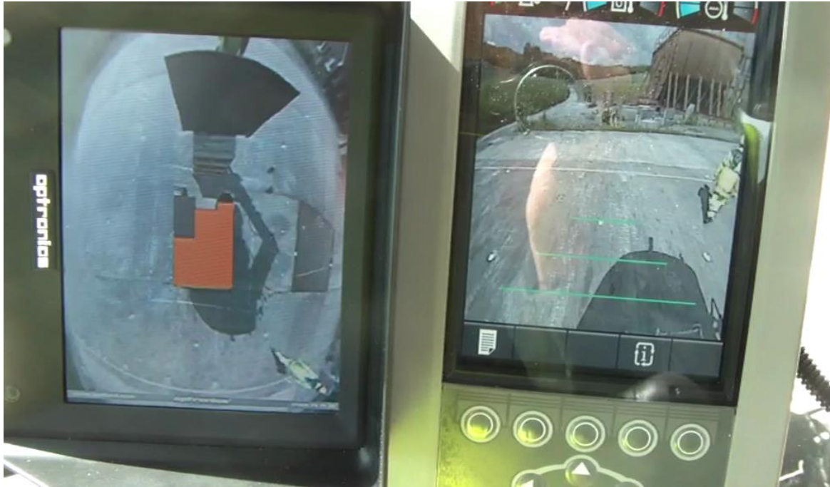
Photograph 7 Example of the monitor screen for a surround-view camera system (left) and conventional rear view camera system (right) fitted to an excavator (SDV_0428 (2:03))
