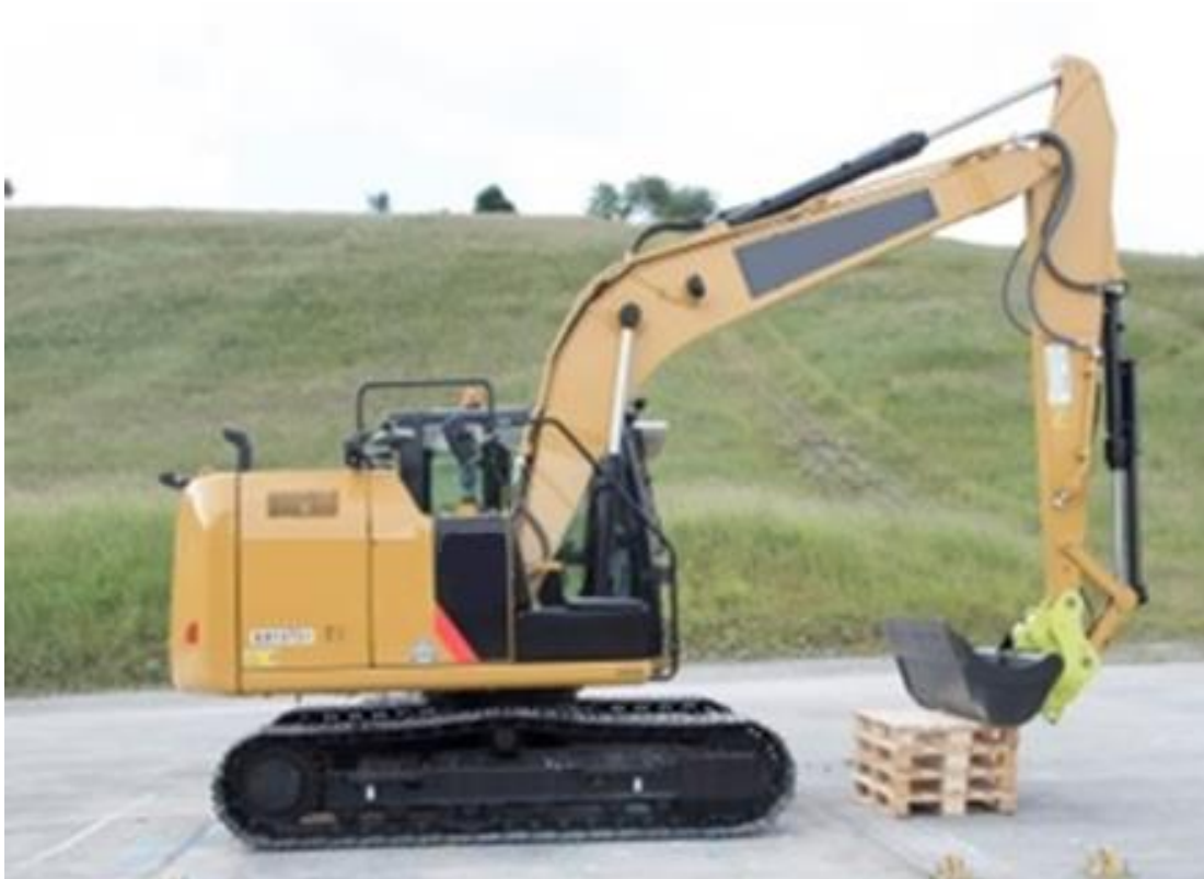
Photograph 4 Travel position of the hydraulic excavator included in the trial of the visibility risk zones method
