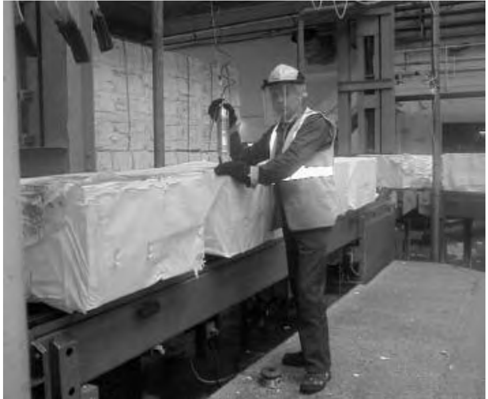
Figure 10 Pneumatic cutters are easier to use than manual cutters
