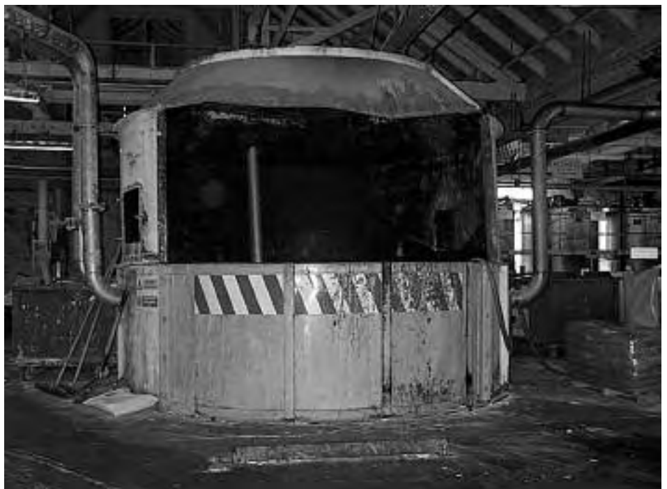
Figure 13 The fencing around open-topped pulpers should be designed so that people cannot climb onto it
