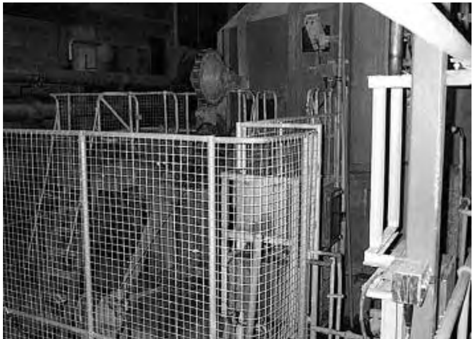
Figure 15 Ensure the guard is interlocked with both the movement of the capstan and the pneumatic system for operating the guillotine
