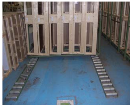
Photograph 6. Rollers used to help transport divan bases
