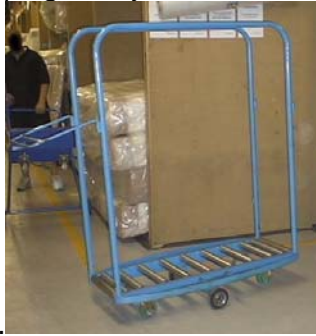
Photograph 3. Examples of specialised trolleys to transport mattress (a&b) and fabric rolls (c)
