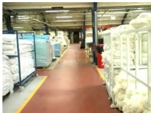
Photograph 11. An example of a clearly marked walkway with products stored in large trolleys so they can easily transported within the factory
