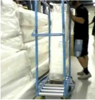
Photograph 3. Examples of specialised trolleys to transport mattress (a&b) and fabric rolls (c)
