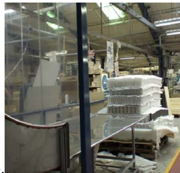
Photograph 4. The chute where mattresses are delivered from the upstairs production area (a) and the end of the chute on the ground level (b)
