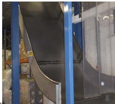
Photograph 4. The chute where mattresses are delivered from the upstairs production area (a) and the end of the chute on the ground level (b)
