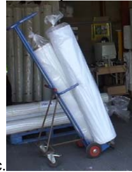
Photograph 3. Examples of specialised trolleys to transport mattress (a&b) and fabric rolls (c)
