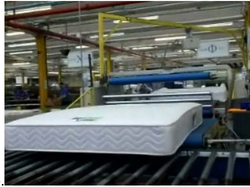
a. Photograph 34. Mattress leaving the mattress turner and moving onto the conveyor system
