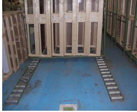
Photograph 40. Rollers used to help transport divan bases
