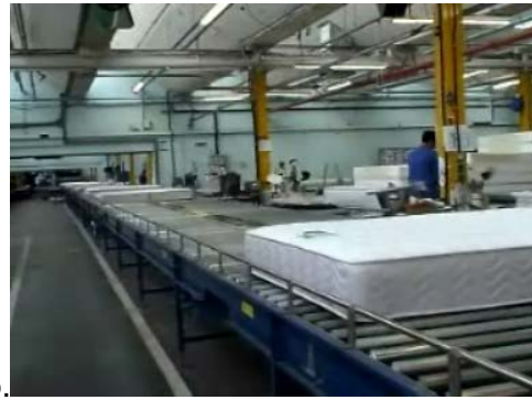
Photograph 32. Examples of different types of conveyors used along the production line
