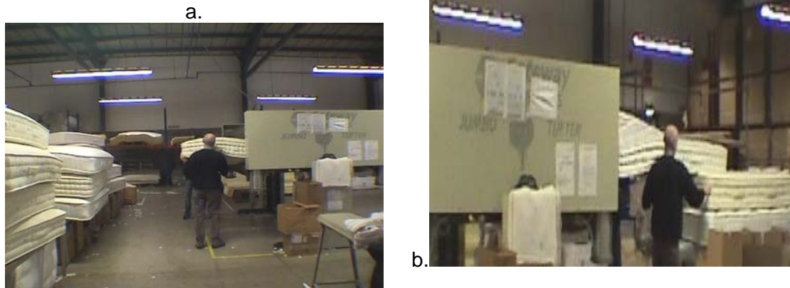
Photograph 13. Lifting into and out of a tufting machine
