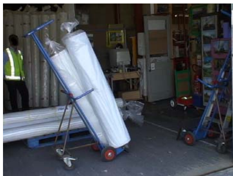
Photograph 42. Specialised trolleys to transport fabric rolls
