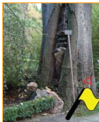
Conks and bark damage around a cavity in Celtis – The stem of this Celtis would not have had sufficient strength to withstand an estimated wind load at speed 12 Beaufort, according to results of a pulling test (Elasto-Inclinomethod).
