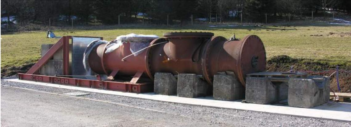
**Figure 3: General view of 1.04 m diameter pipe vessel and target support frame (6 m length shown)**
