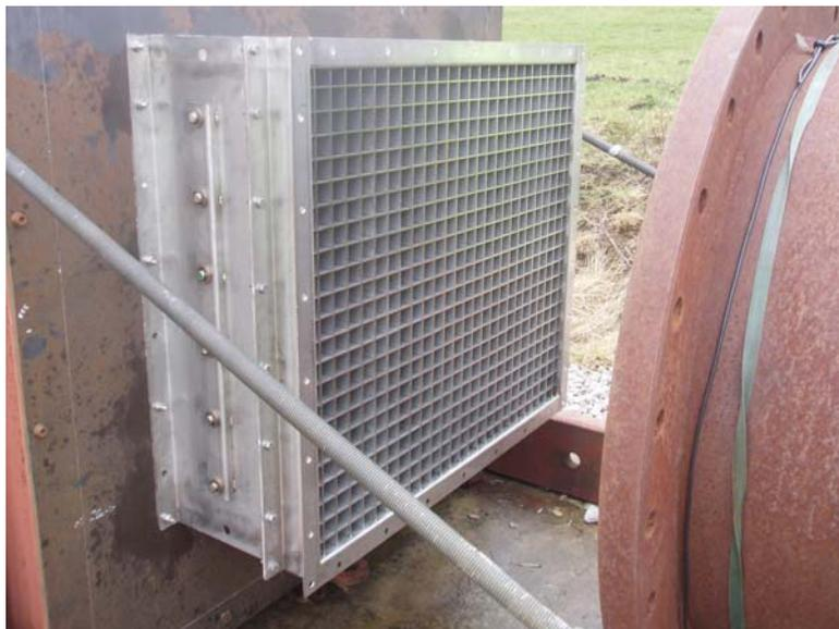
**Figure 9 The damper mounted ready for the blast test. The diffuser attached to the front of the damper can clearly be seen.**
