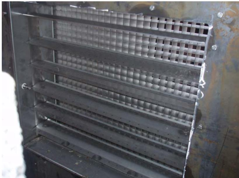
**Figure 14 A view of the open damper post-test. The damper behaved normally during this test.**
