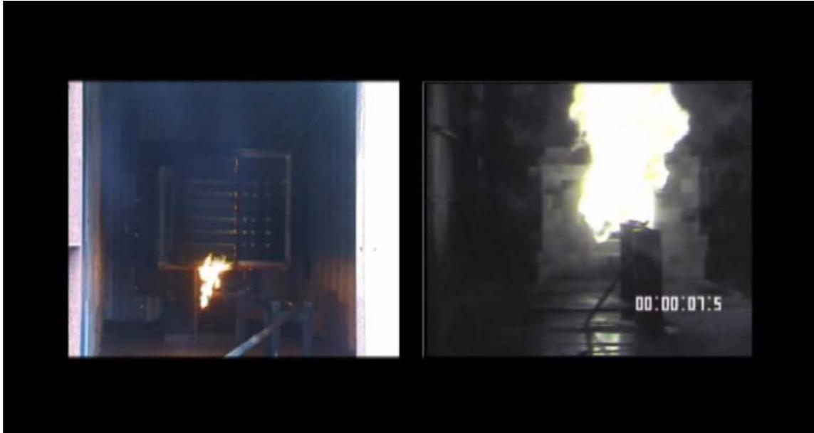
**Figure 19 Simultaneous front and rear views of the jet fire test taken after 7.5 s. The enveloping flame of the jet fire can be clearly with no penetration of flame into the ducting.**
