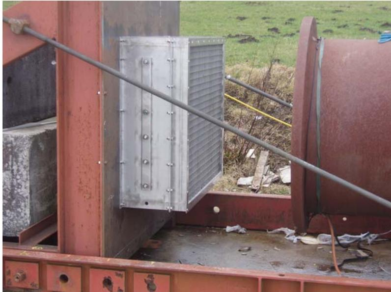
**Figure 10 The damper in position ready for the blast test, showing its position relative to the open end of the pipe.**
