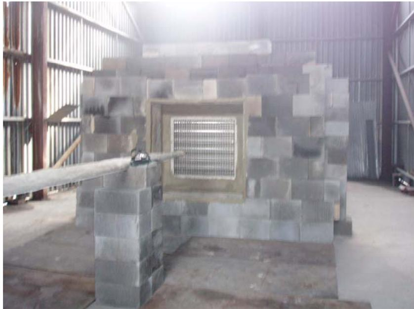
**Figure 18 The damper installed in the test building with the surrounding blockwork wall. The fuel supply pipe for the jet fire can be seen running from the left to the centre of the photograph.**
