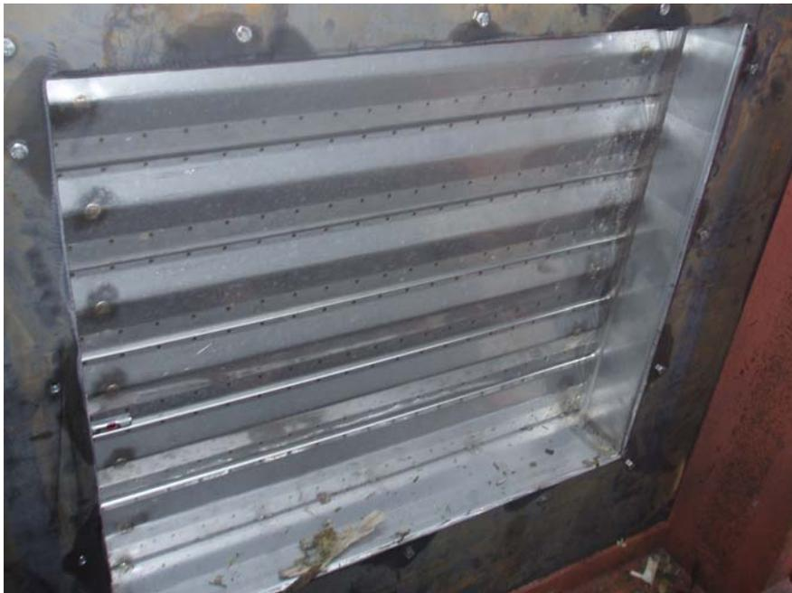
**Figure 12 A general view of the rear of the damper post-test**
