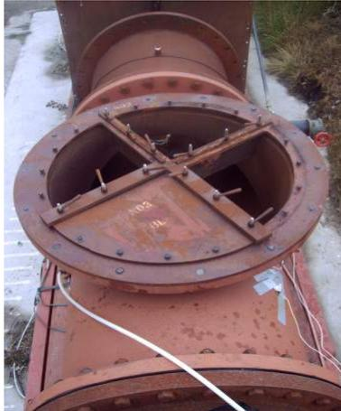
**Figure 5: Removable vent panel arrangements (3/4 open)**
