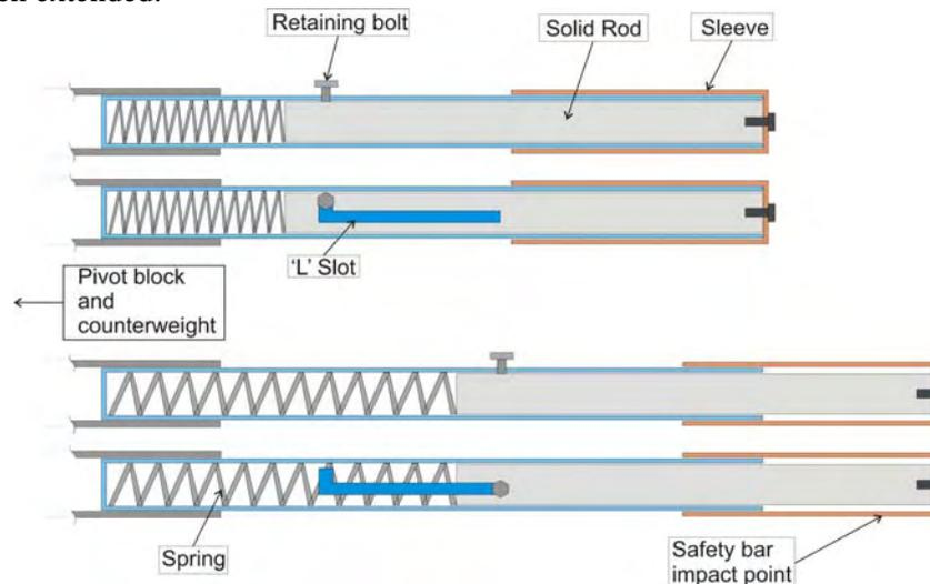
**Figure 3** Operation of the spring loaded trigger arm
