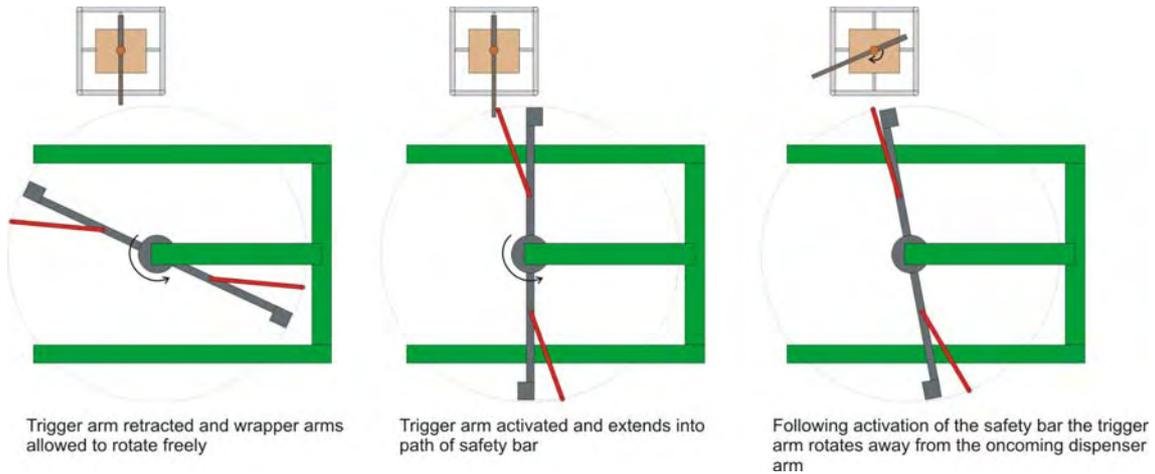
**Figure 4** Operation of test rig
