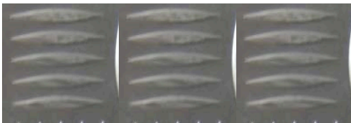
Figure 3.3 All ridges parallel with direction of travel of the slider, calculated PTV = 26 in water-wet conditions
