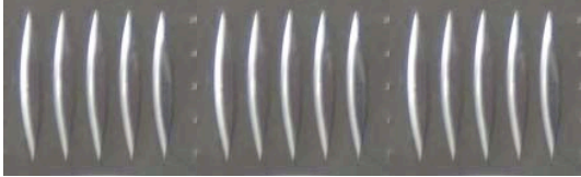
Figure 3.3 All ridges parallel with direction of travel of the slider, calculated PTV = 26 in water-wet conditions
