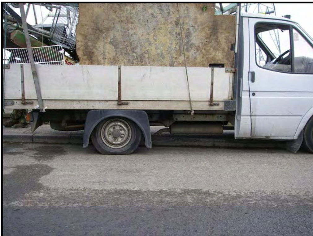
Photo 3: A different angle of the vehicle shown in Photo 2 illustrating that the vehicle is also overloaded.
