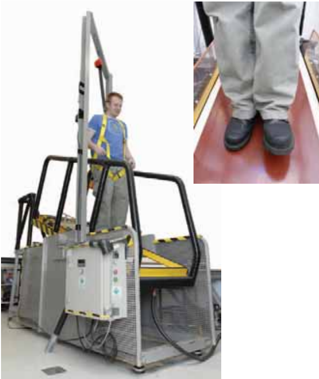
Figure 4 The UKSRG ramp CoF test
