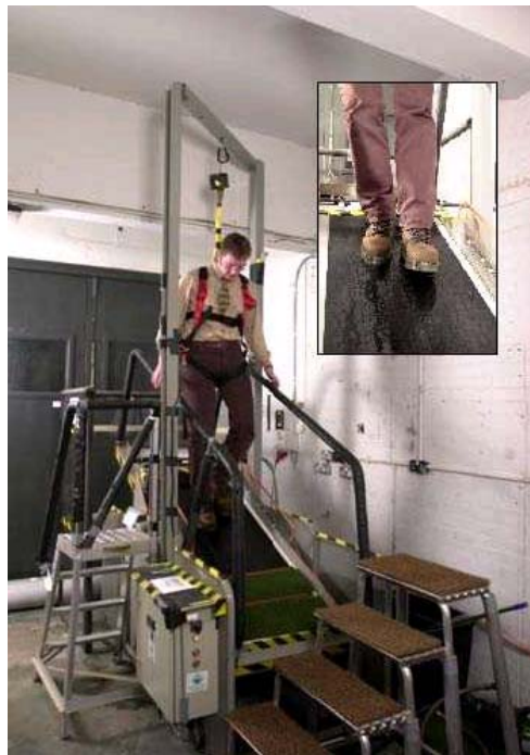
Figure 2.3: The ‘HSL-PS-SOP-12’ ramp CoF test.
