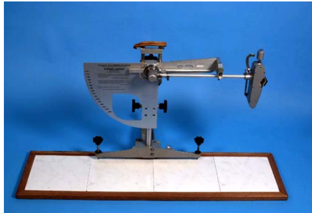
Figure 2.2: The “Stanley” Pendulum CoF test.
