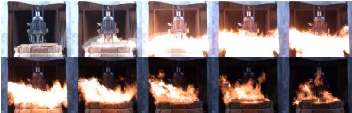
Figure 9 Frame grabs from the video of ignition test Ink 3: ink with ethanol and ethyl acetate as solvents. Timebase: 25 fps, frame numbers, 0,2,3,5,6,8,10,12,14,16 Picture width inside blue framing 2.180 m Picture height inside blue framing 1.875 m
