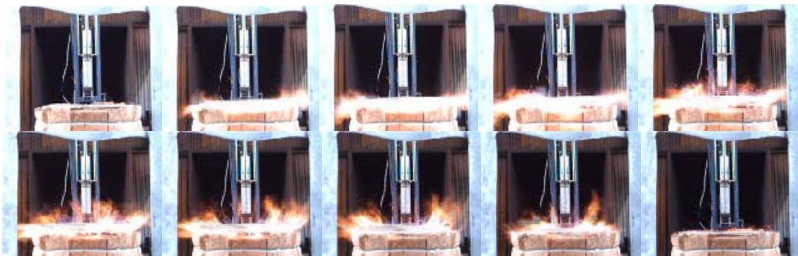
Figure 7 Frame grabs from the video of ignition test Ink 1: ink with ethanol and ethyl acetate as solvents. Timebase: 25 fps, frame numbers, 0,2,3,4,5,6,7,8,9,11. Picture width inside blue framing 2.180 m Picture height inside blue framing 1.875 m
