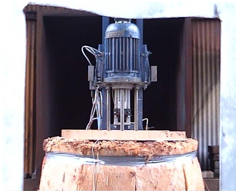
Figure 6 A frame grab from the video of ignition test Paint 1: paint with xylene as the solvent. Picture width inside blue framing 2.180 m Picture height inside blue framing 1.875 m
