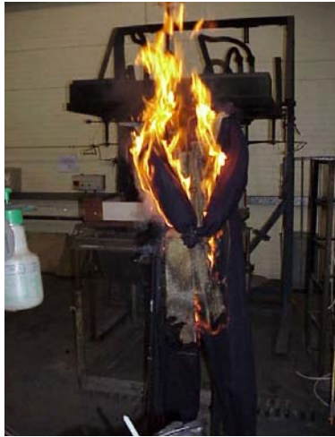
Figure 2. Grinder sparks have been applied to a manikin (non-FR boiler suit). The result after approximately 45 seconds (ignition occurred at approximately 20 seconds).
