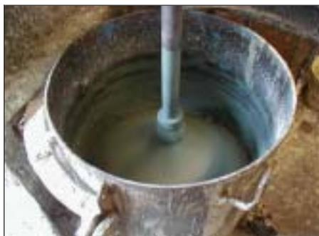
**Figure 15 - Mixing Drum**
