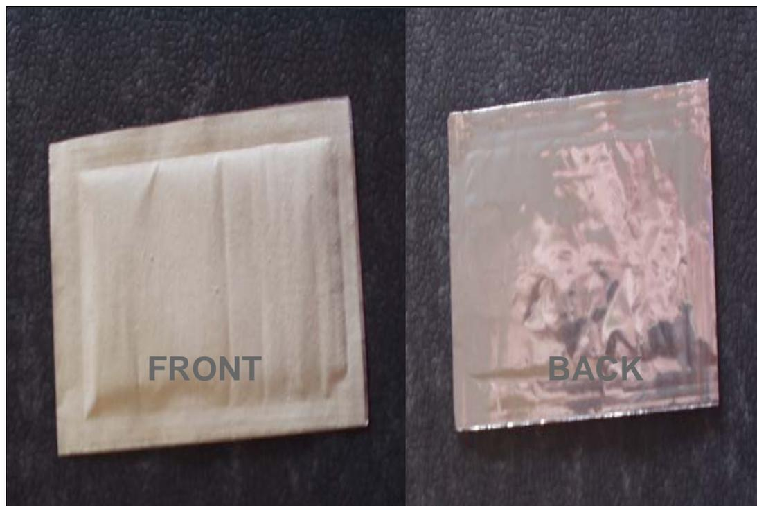
**Figure 6 - Pictures of the prototype, illustrating the diffusive membrane on the front and the laminated foil on the back**
