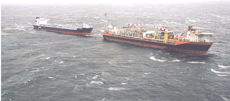
Figure 1 Example of FPSO and shuttle tanker configuration
