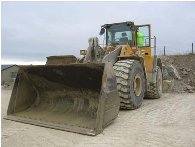
**Figure 2** Example of a loading shovel
