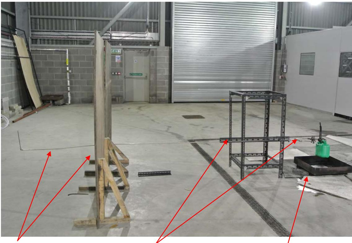
Operator adjustable arm and protective shield. Arm support and fuel container clamp. Fire tray.
