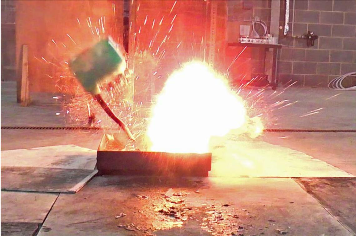
Figure 4 - Explosion with 1.5 ml petrol
