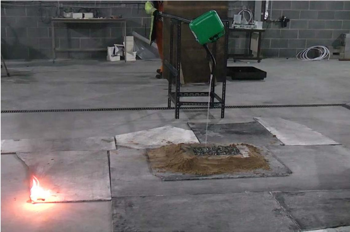
Figure 7 – Demonstration of pouring petrol near a naked flame, note the flame is straight as there is no noticeable draught
