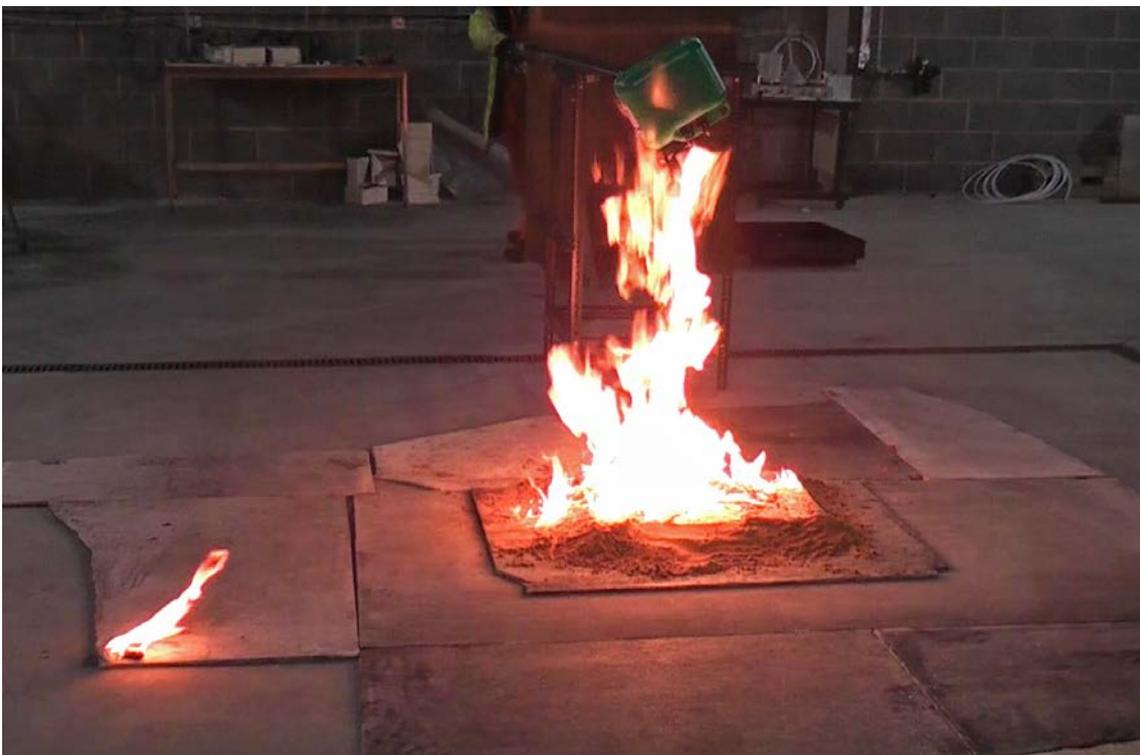
Figure 10 - After 21 seconds from commencement of pouring, the petrol is now alight
