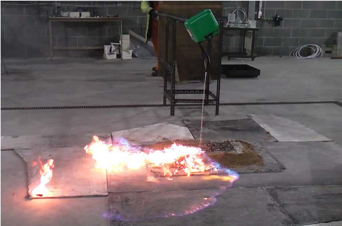
Figure 9 - Flames travel across the vapour towards the source of pouring
