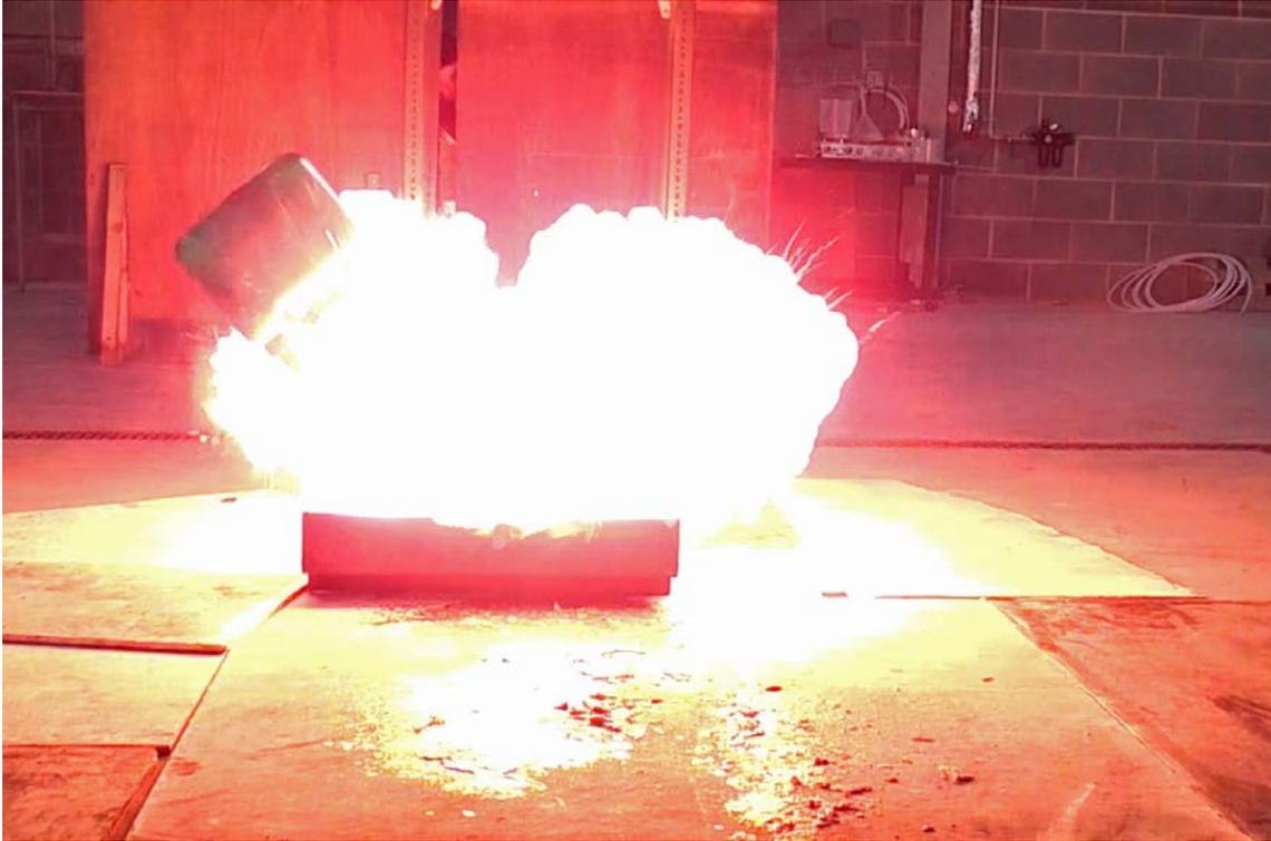
Figure 6 - Explosion of 100 ml of toluene as burning liquid is ejected from spout.
