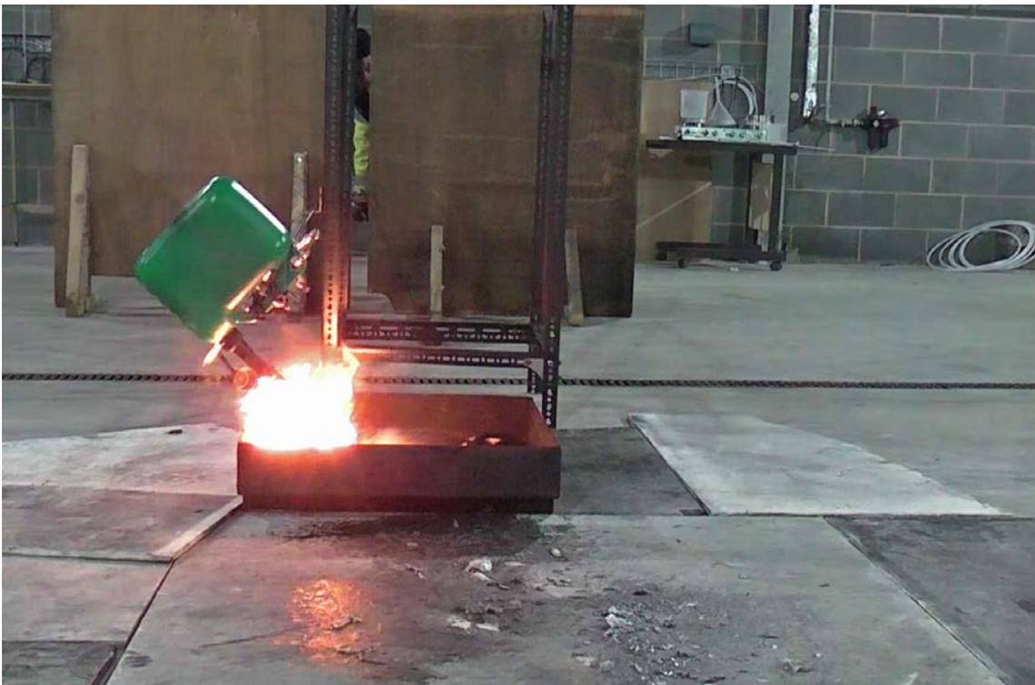
Figure 5 - Start of explosion with 100 ml toluene
