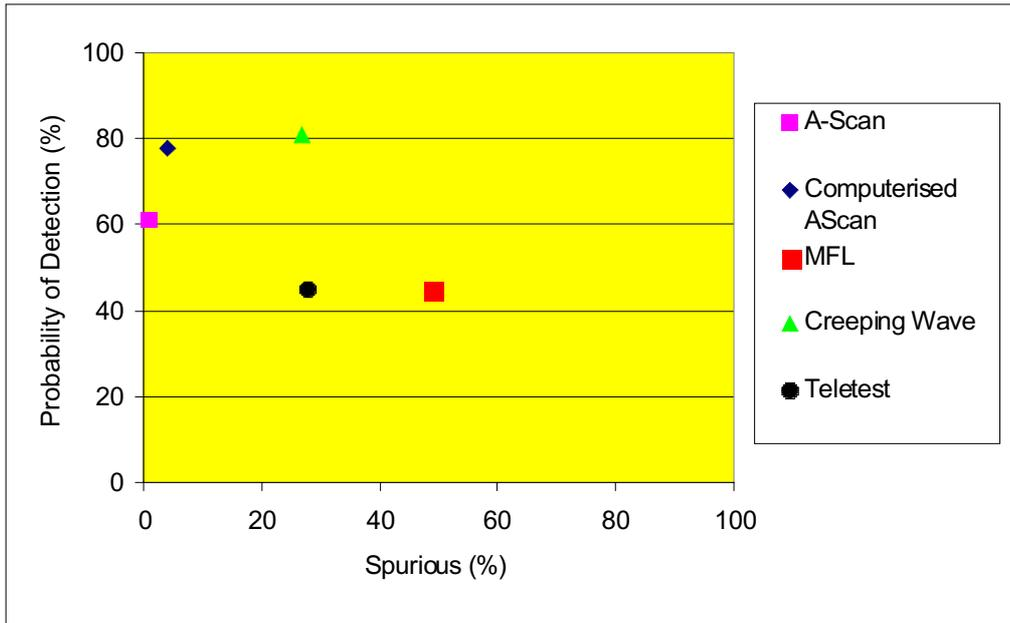
Figure 16 Reliability Operating Characteristic(ROC) for bare Steel Cumulated Thickness
