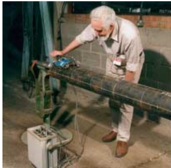
Figure 2 MFL Pipescan in RACH Trial
