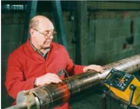
*Figure 1 A-Scan equipment in RACH Trial*
