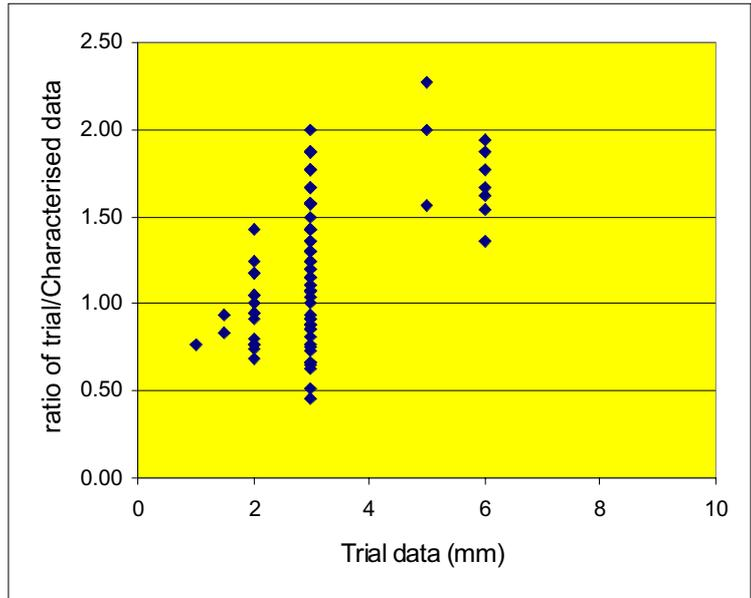
Figure 12 CHIME Tested on Bare Steel Cumulated Thickness
