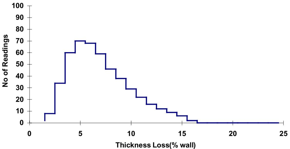
Figure 24 Example of high resolution wall thickness readings
