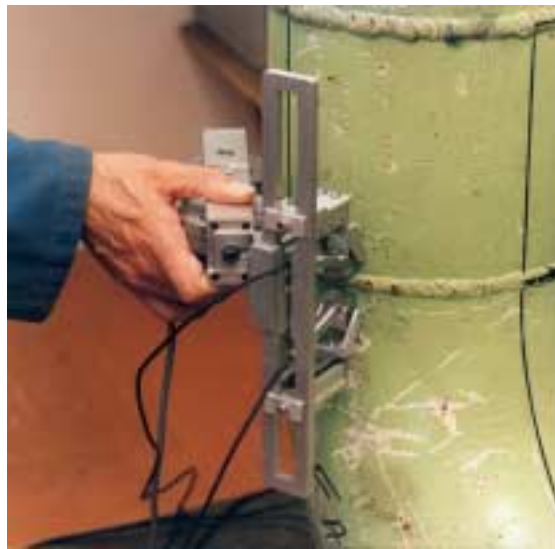
Figure 8 TOFD RACH Trial
