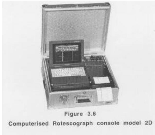
Rotesco has also completed the development of the computerised Rotescograph console, Model 2D, shown in figure 3.6, above. The computerised Rotescograph incorporates a Notebook computer which controls the instrument and stores the data. The standard test heads cover the range of rope sizes between  $\varnothing 6$  mm and  $\varnothing 63.5$  mm, with specialist heads available outside this range.
