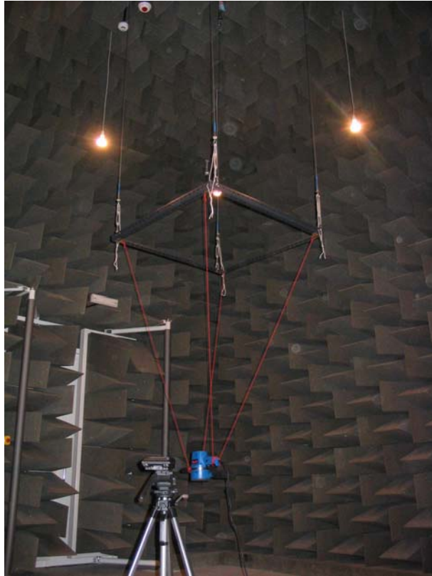
Figure 4. Test rig for electric sanders & polishers (and pneumatic polishers)
