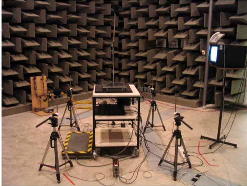
Figure 2. Test rig for pneumatic sanders
