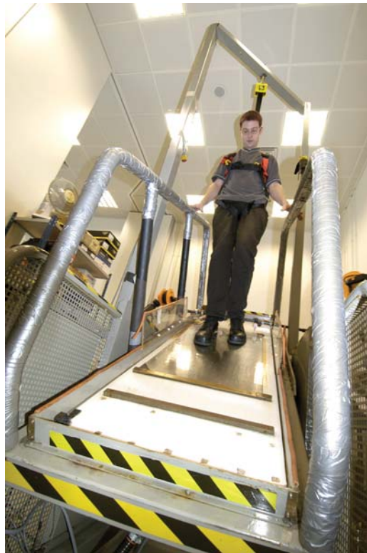
Figure 2.4. The 'HSL-PS-SOP12' ramp-type CoF test.
