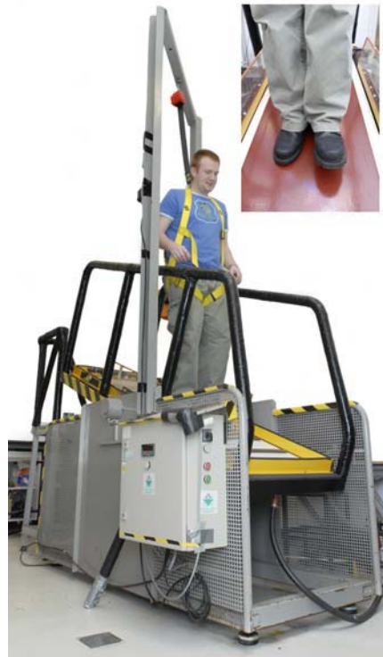
Fig 2.3. The 'HSL-PS-SOP12' ramp-type CoF test.
