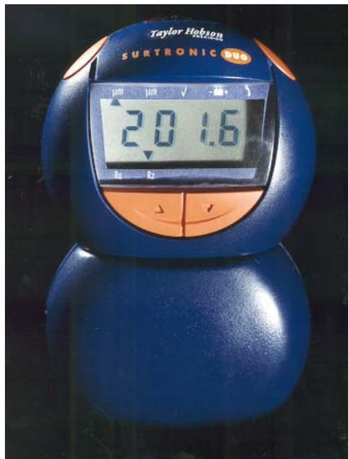
Fig 2.1. The Surtronic Duo microroughness transducer
