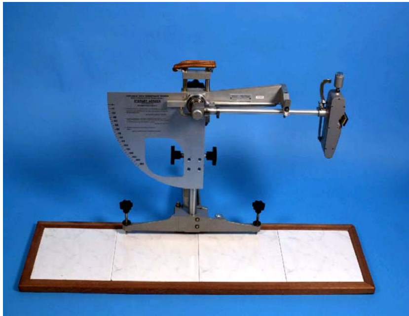
Fig 2.2. The 'Stanley' Pendulum CoF test
