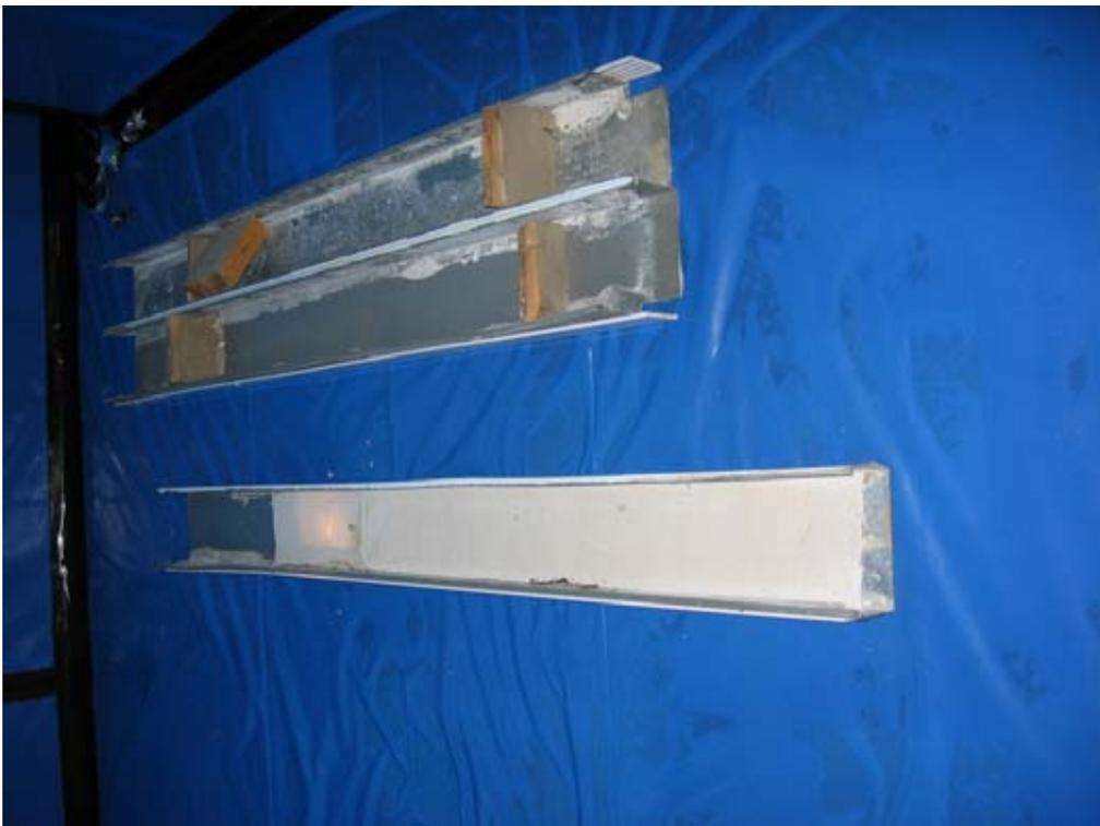
Figure 14: Example of casings removed from columns showing where AIB had been removed or left in place.
