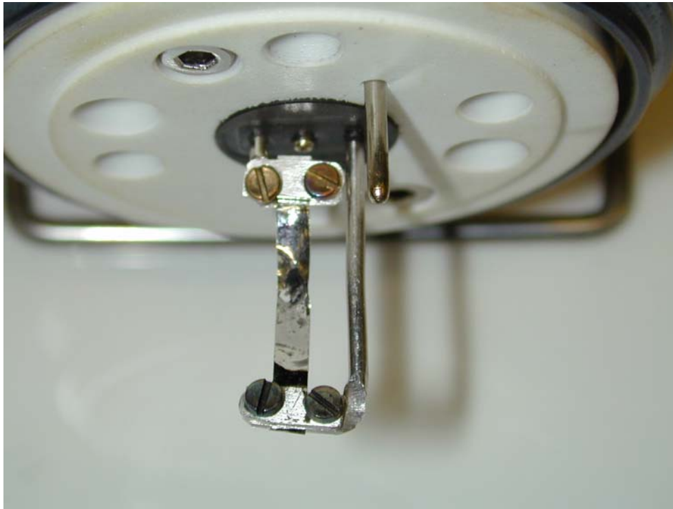
Fig. 2: Pyrola 2000 - Platinum filament and sample
